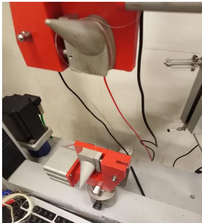
Figure 3. 3: Experimental set up of sisal fiber on the UTM
