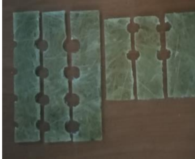
Figure 3. 20: Half Sectioned Samples for Surface Roughness Measurement
