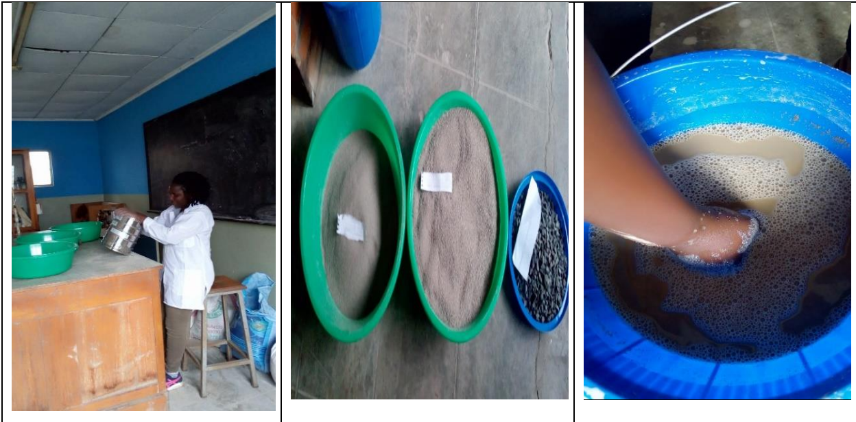
Preparation of local materials for filtration; Sand sieving (left), graded sand and gravel (middle), washing sand (right)
