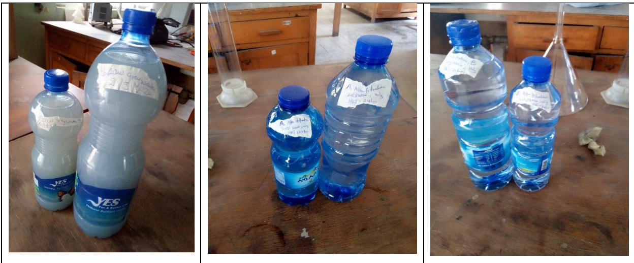
The left is the raw water; middle treated greywater from filter column A; Right is the treated greywater from column B.
