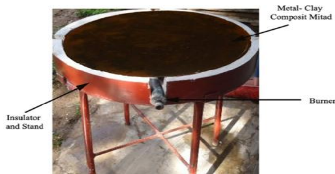
Figure 28. Composite Mitad with Ring Burner
