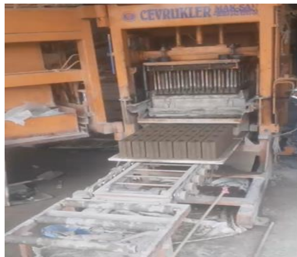
Figure 3. 6: Moulding Machine of hollow concrete block
