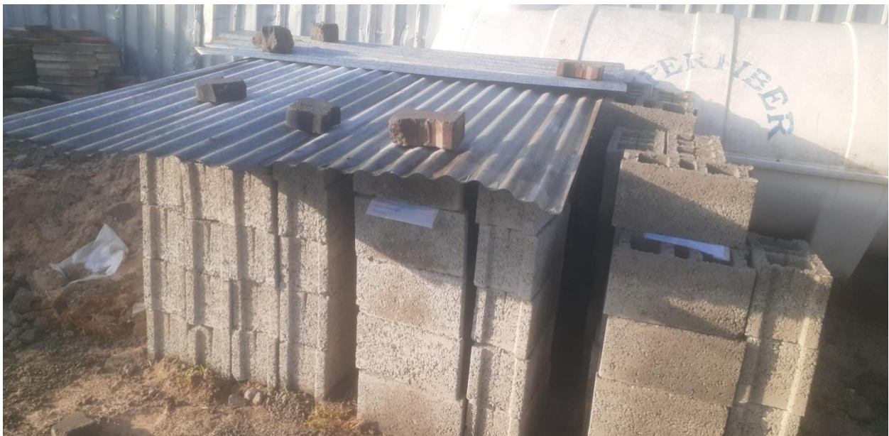
Figure 3.7: Hollow concrete block samples on the production place
