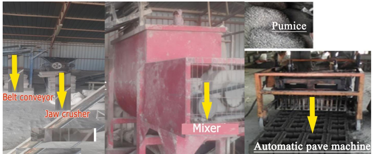
Figure 3. 5: Mixing Machine and mixing process
