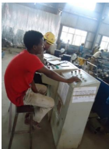
c) Application of prestressing force
