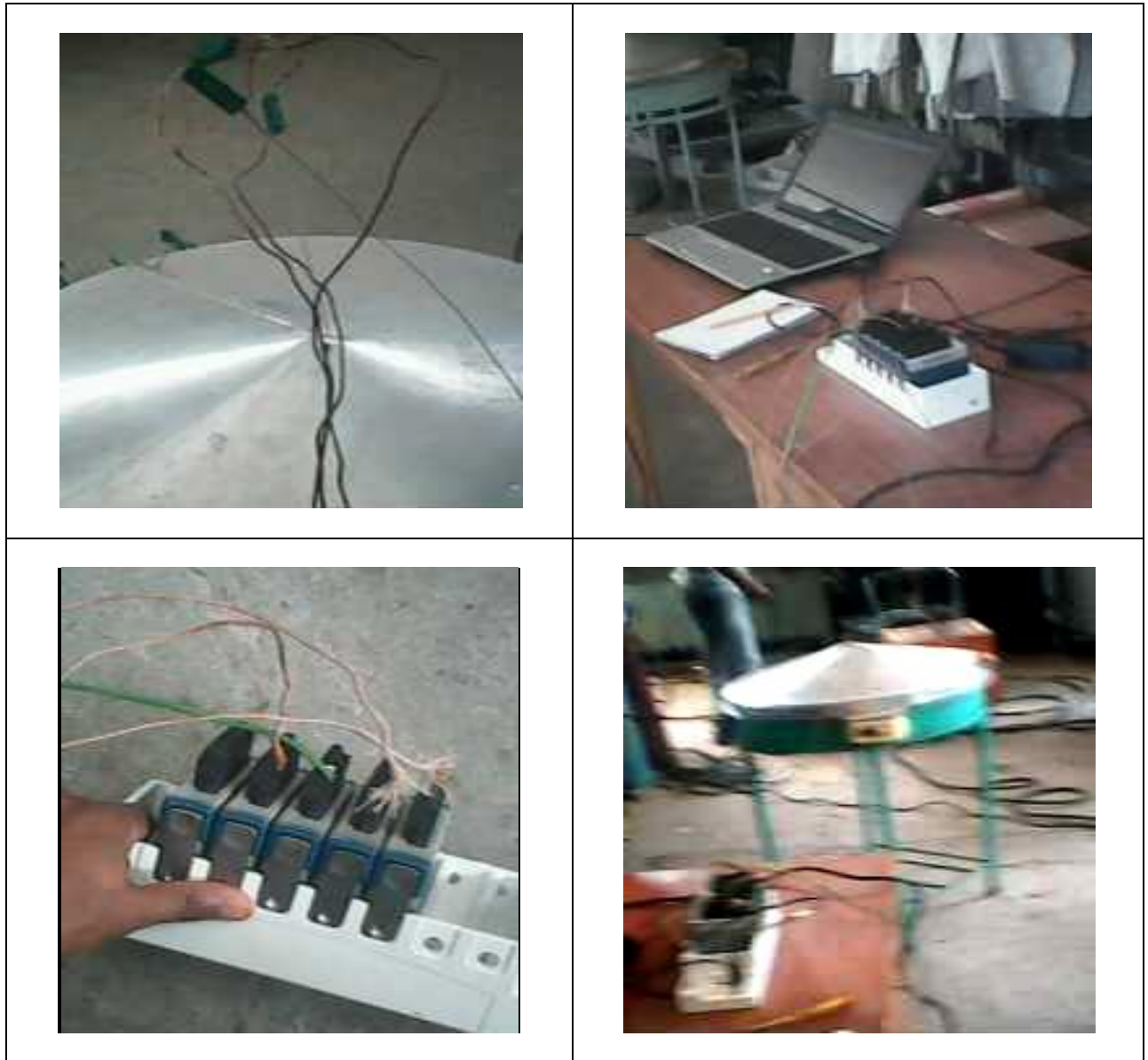
Figure 5.4: Experimental set up of thermocouples during heating up and cyclic injera baking process
