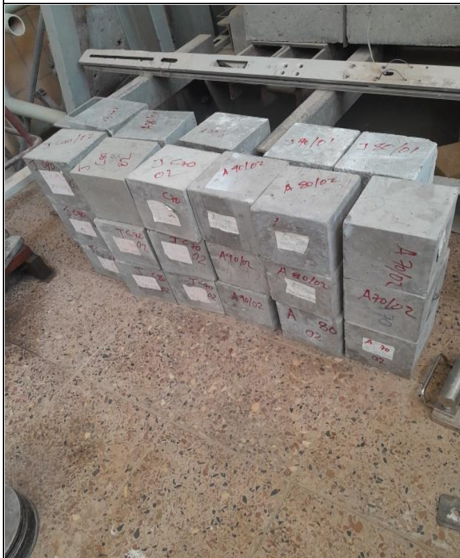
Fig. 7: Concrete cube specimen before testing
