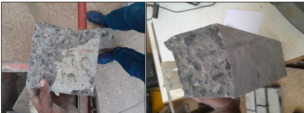
Figure 4. 1: Failure mode of samples (Left: under axial load, Right: under flexure load)
