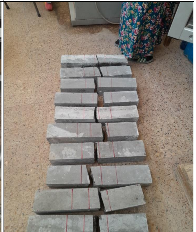
Fig. 8: Flexural bars after test (failure is at the middle third)
