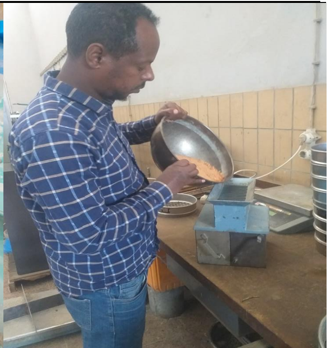
Fig. 6: Quartering of sand before sieve analysis
