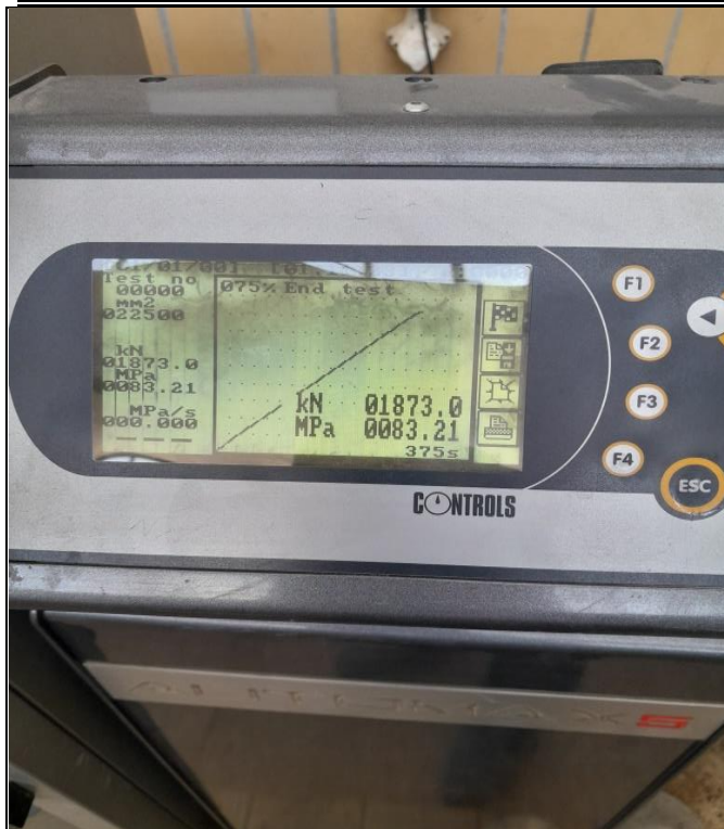
Fig. 9: Typical compressive test reading on the CTM
