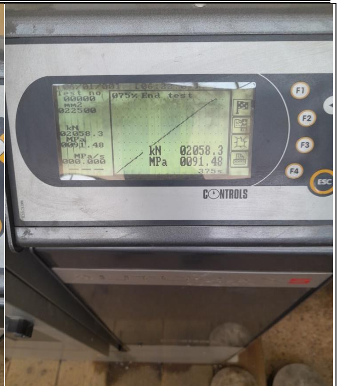
Fig. 10: Typical compressive test reading on the CTM
