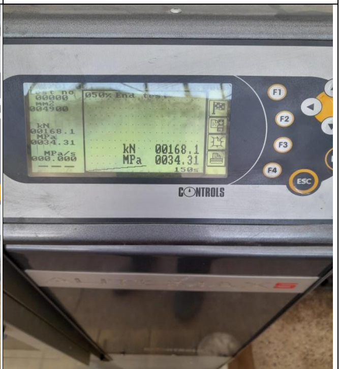
Fig. 12: Typical mortar test reading on the CTM
