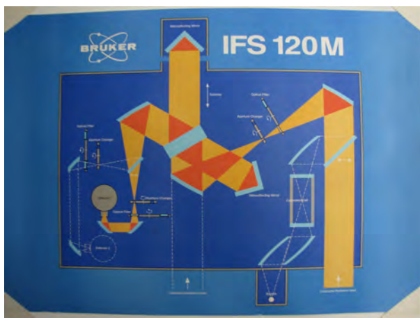
Figure 10.1: Schematic diagram of IFS120M working principle.
