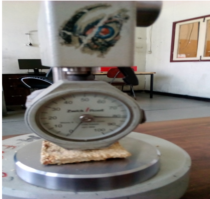
Figure 4.2 Hardness measuring setup of particle board (ASTM Roell, M.FOS.013)
