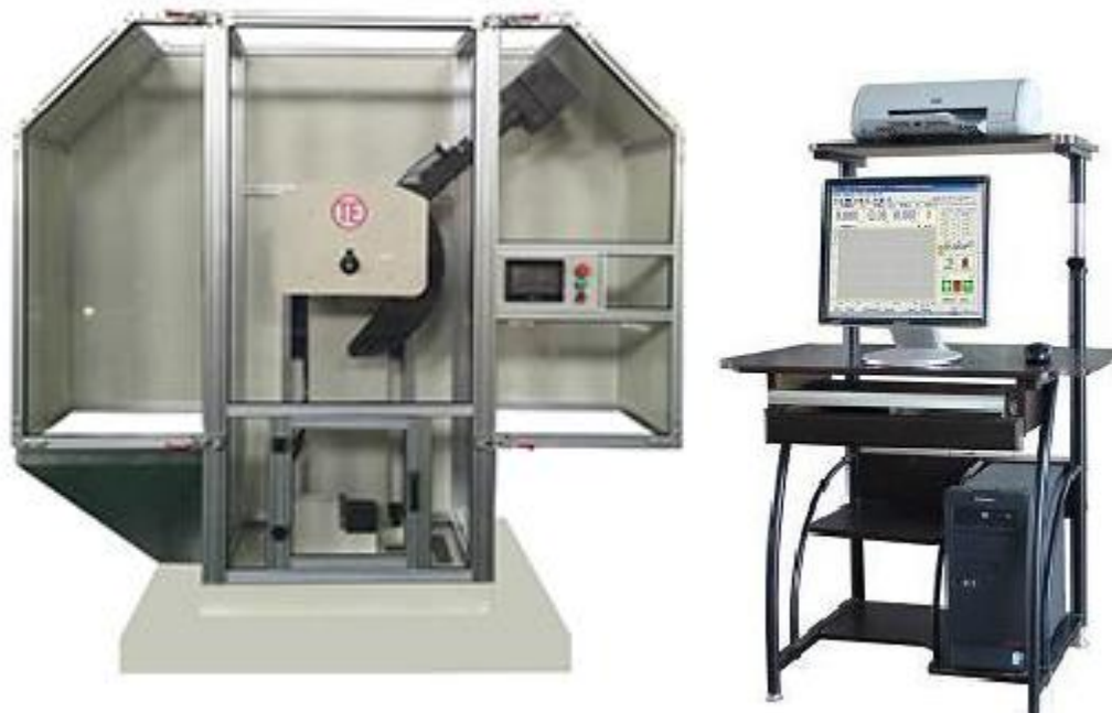
Fig.18 computer integrated Izod impact testing machine model JWT 406
