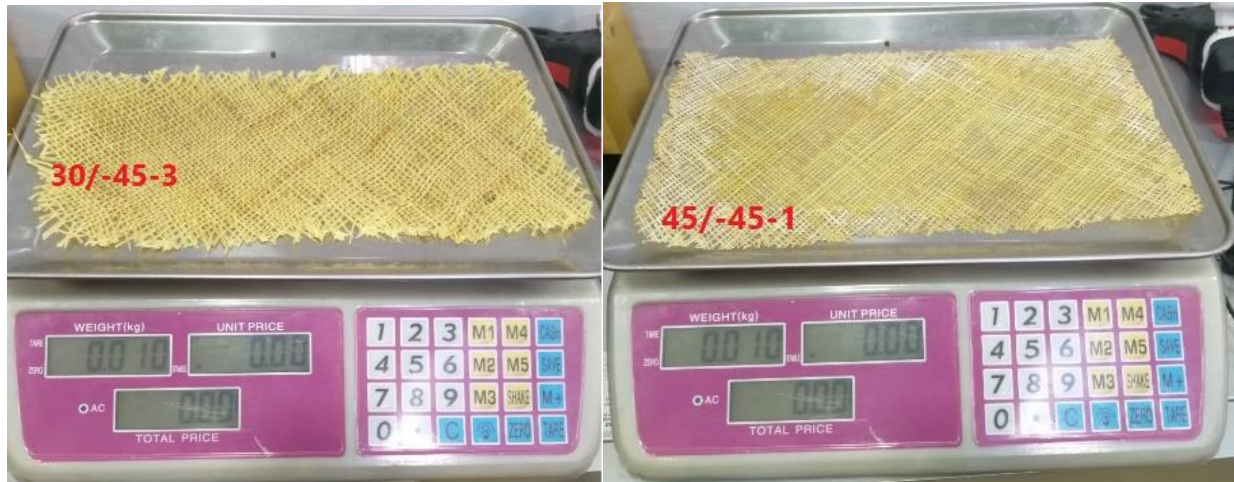
Fig. 8 mass of 30 0 /-45 0 (left) and 45 0 /-45 0 (right) woven sisal fiber plies
