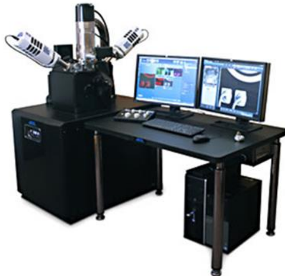
Fig. 17 SEM model: JSM-IT300LV Scanning electron microscope set up (LDI) laboratory
