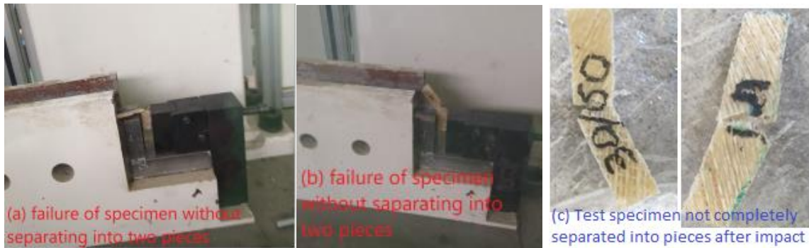
Fig. 25 breakage of the test specimen which the fiber bundle holds the two pieces together
