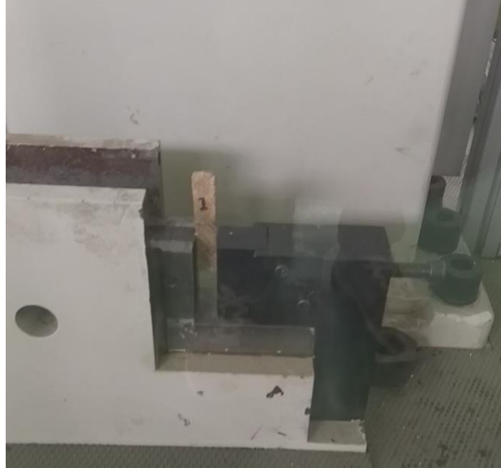
Fig. APPEX 3 B1 A45 0 /45 0 specimen number one clamped on Izod anvil
