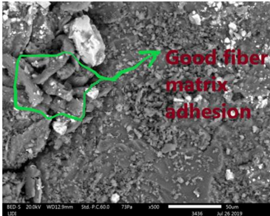
Fig. 30 A 45 0 /-45 0 WSFRUPC 100μm SEM micrograph
