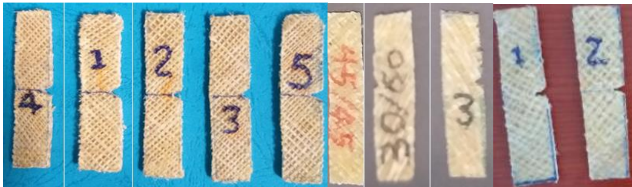
Fig. 16 Test specimens cut and notched according to ASTM D256
