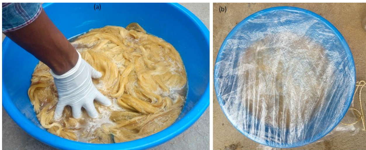
Fig. 6(a) washing sisal fiber with 5% NaOH solution, (b) Sealing sisal fiber immersed in 5%NaOH solution (2Hrs)
