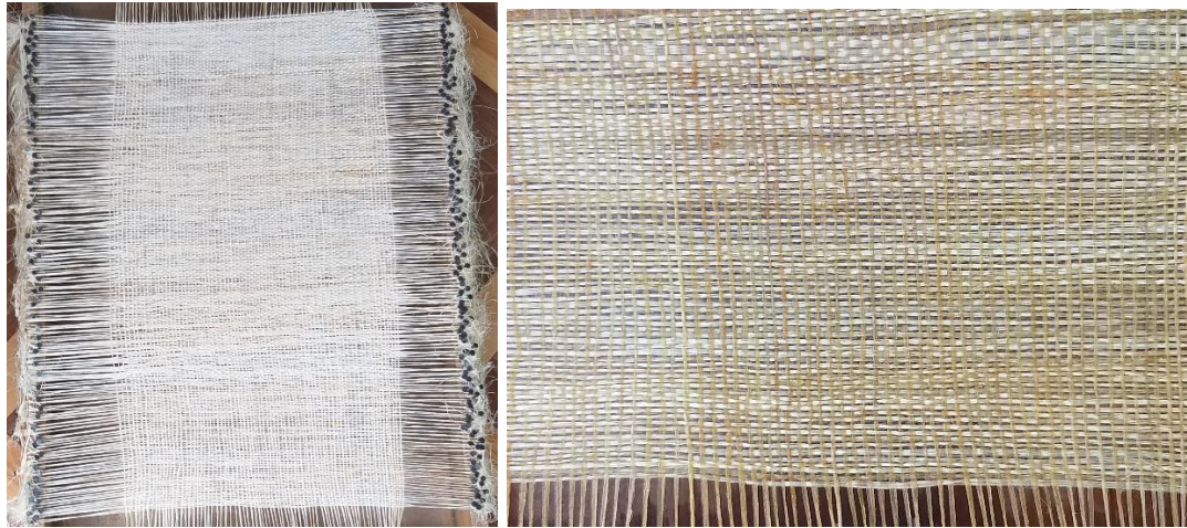
Fig. 9 wooden frame for wrap &weft guiding (a) before woven ply preparation (b) after woven ply preparation
