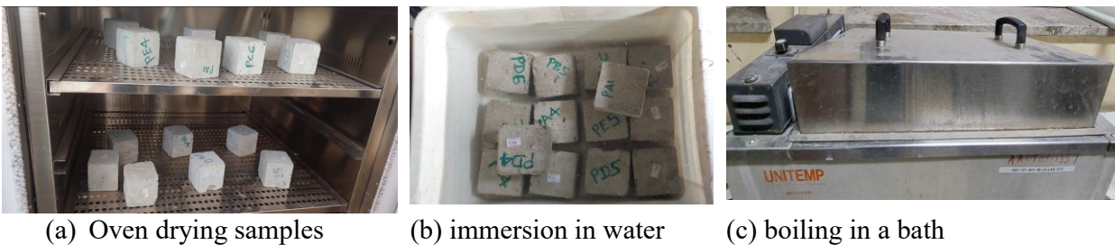
Figure 3.14. Volume of voids and absorption examination
