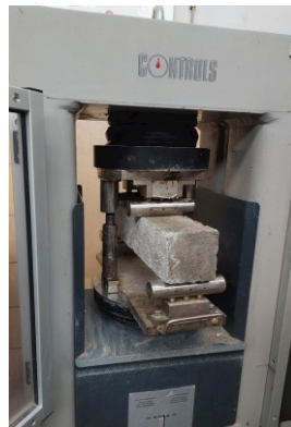
Figure 3.8. Set up for flexural strength
