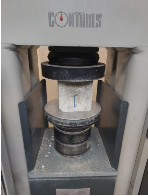
Figure 3.6. Compressive strength machine
