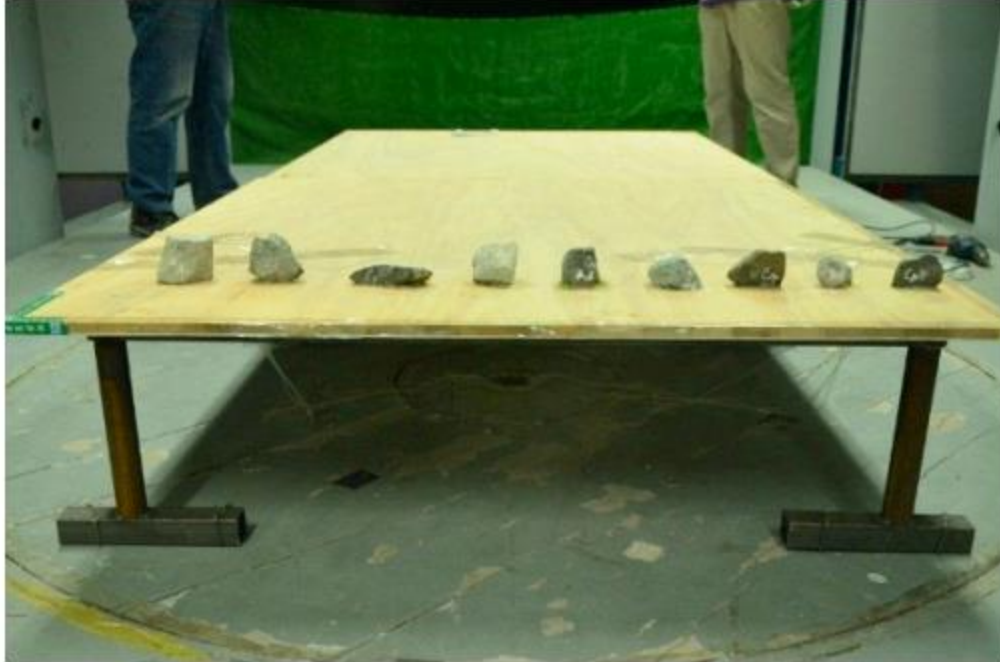
Figure 2.4: Laboratory wind tunnel test to measure critical wind velocity and displacement of ballast [2]
