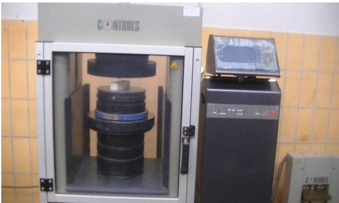
Fig.3. 9 Compressive strength testing
