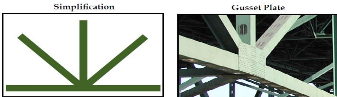
Figure 4.7: Simplification of gusset plate joint
