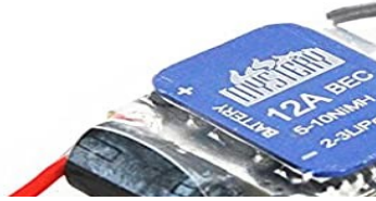
Figure A2: 11.1V, 12 A BLDC motor drive circuit
