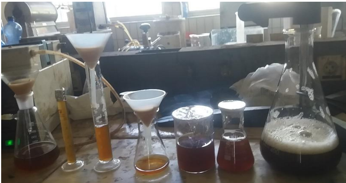
Crude filtered saponin using qualitative filter paper with the aid of vacuumed pressurized machine
