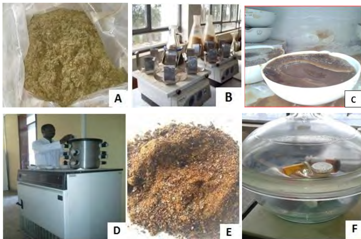
Figure 6:- Photographs showing different steps used in the preparation of the aqueous extracts from the dried plant leaves that has been processed through. (A) Dried powder leaf. (B). On orbital shaker for shaking (C) Freezing, (D) The lyophilizer, (E) The final extract, (F) The desicator.
