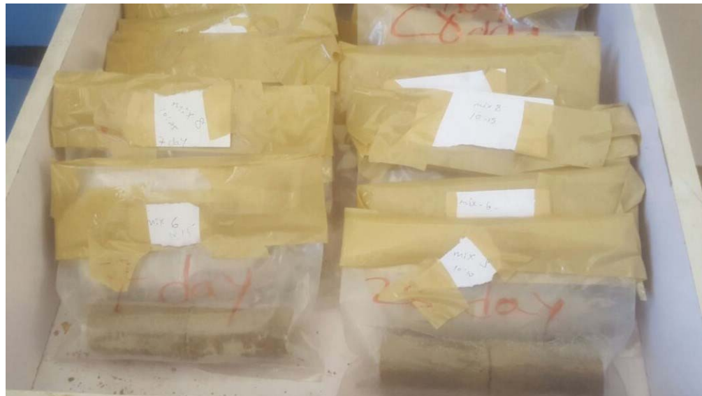
Figure 5-8 UCS samples compacted and cured in moisture proof bags for 7 and 28 days
