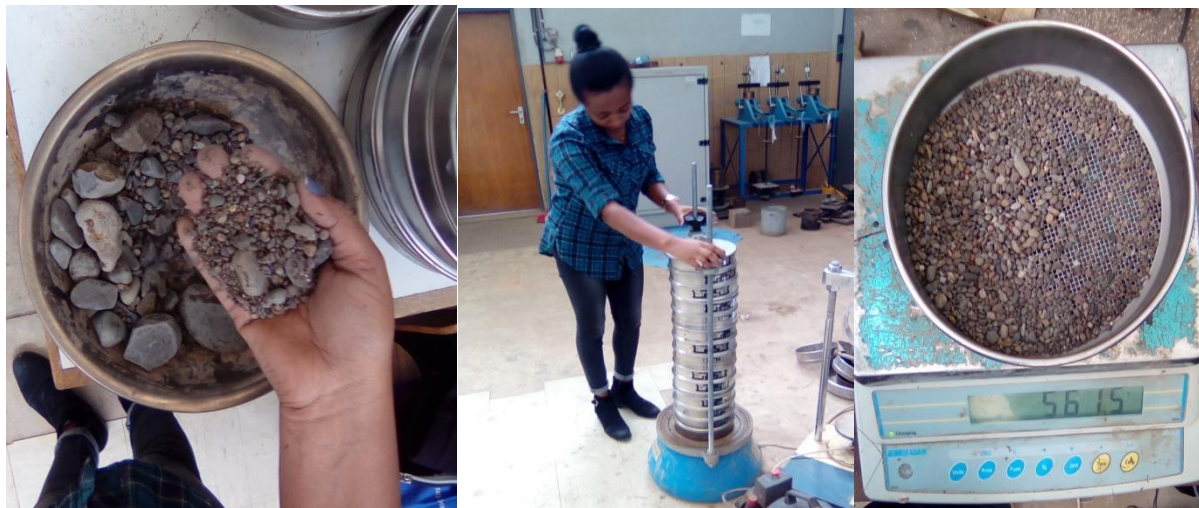
Figure 4-3: Sieve Analysis of Grain size distribution of River bed and River Bank channel at Addis Ababa institute of Technology soil lab (April 02, 2018).
