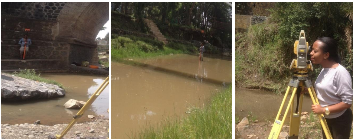
Figure 4-2: Surveying of Ginchi Awash River cross section data (April 02, 2018).
