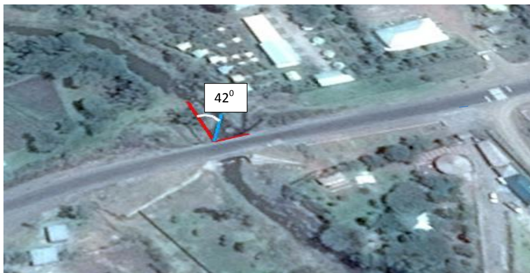
Figure 4-6: Skew angle and Bridge abutment alignment with respect to the flow direction.
