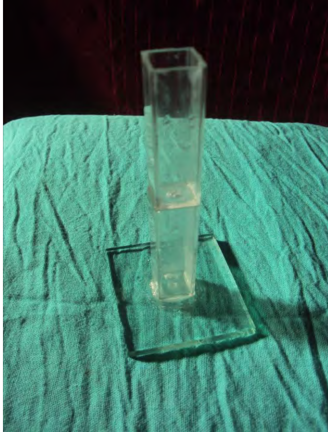
Figure 21 The diffusion cell (made of two cuvettes).
