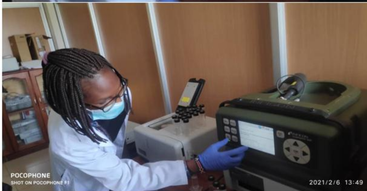
Figure 7.15: Operating a HS Coupled with P& T GC-MS to Measure Trihalomethanes in Drinking Water.
