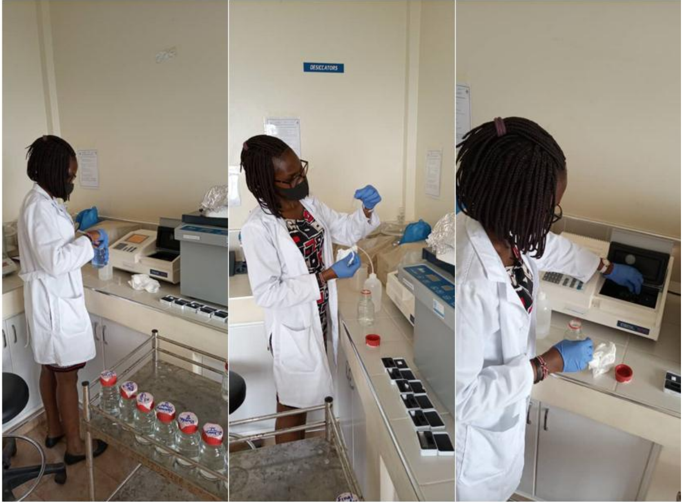
Figure 7.17: Operating the Cecil Spectrophotometer to Measure UV 254 in Drinking Water
