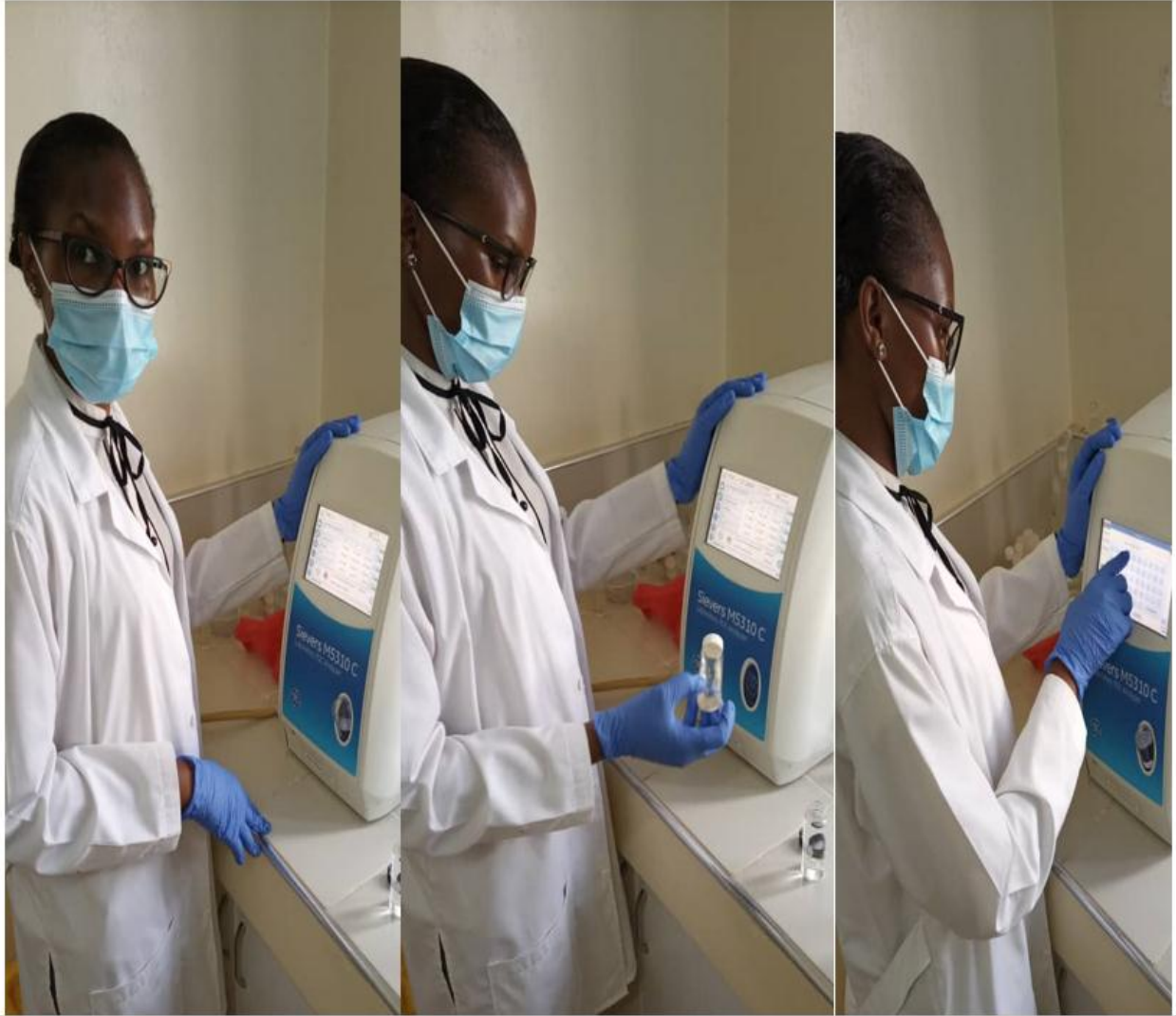
Figure 7.16: Operating Total Organic Carbon Analyzer to Determine TOC in Drinking Water.
