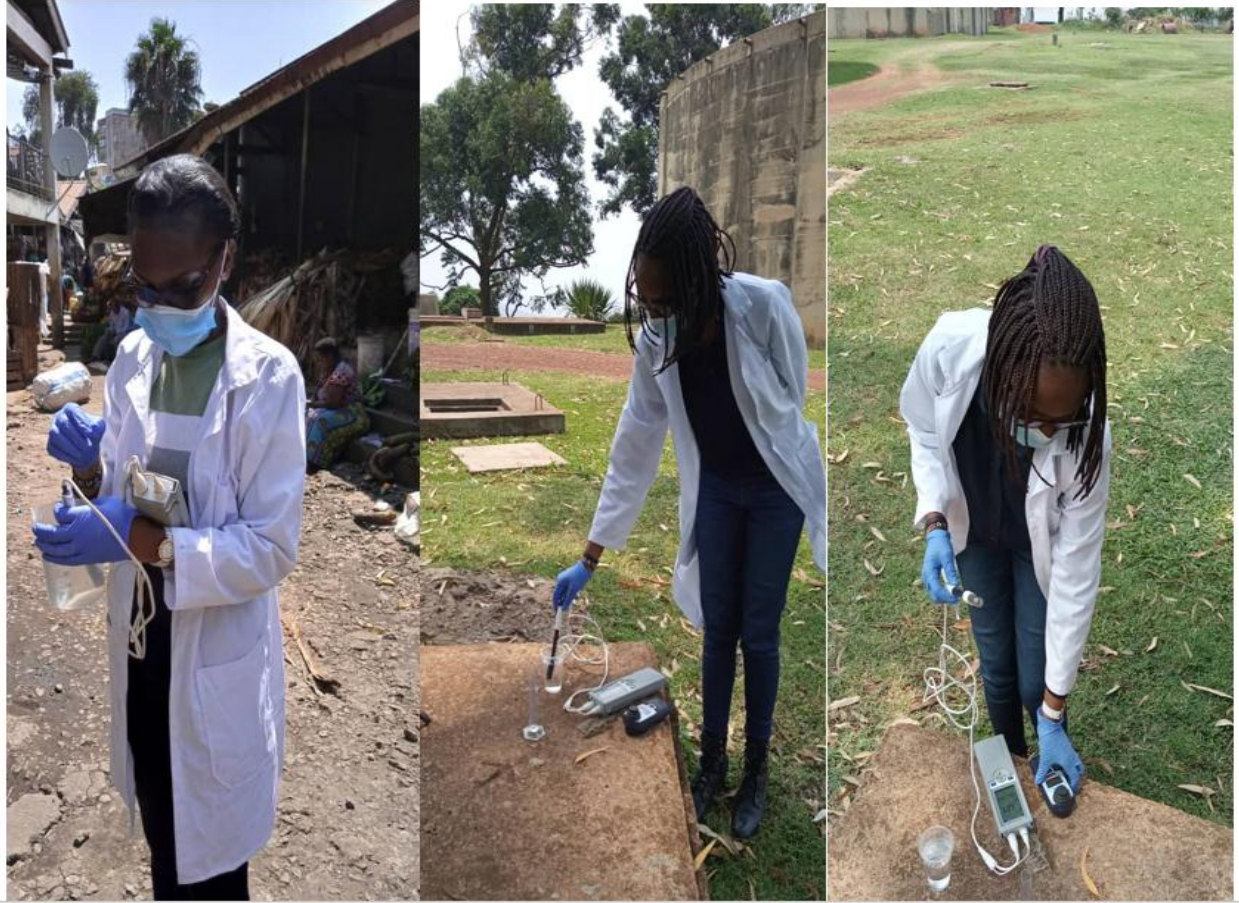
Figure 7.19: Operating a pH meter to Measure pH and Temperature in Drinking Water
