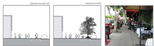
Figure 2.9. The role of street furniture in walkway enclosure. ( LA-Walkability Checklist, 2008:10)
