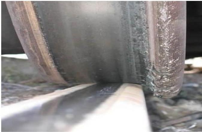
Figure 3.4: wheel/rail contact interface (17)
