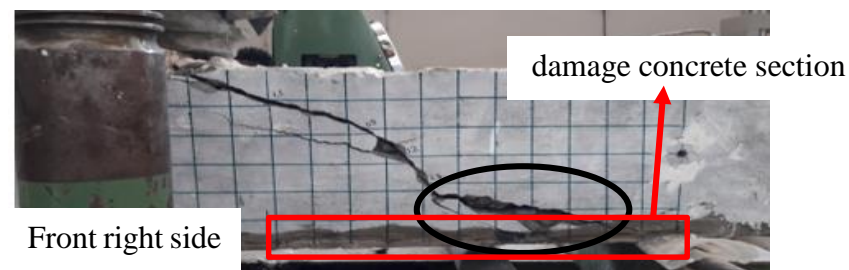
Figure 5-48 Beam 75DCB1 critical diagonal crack
