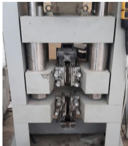
Figure 3-31 Steel mechanical property testing machine
