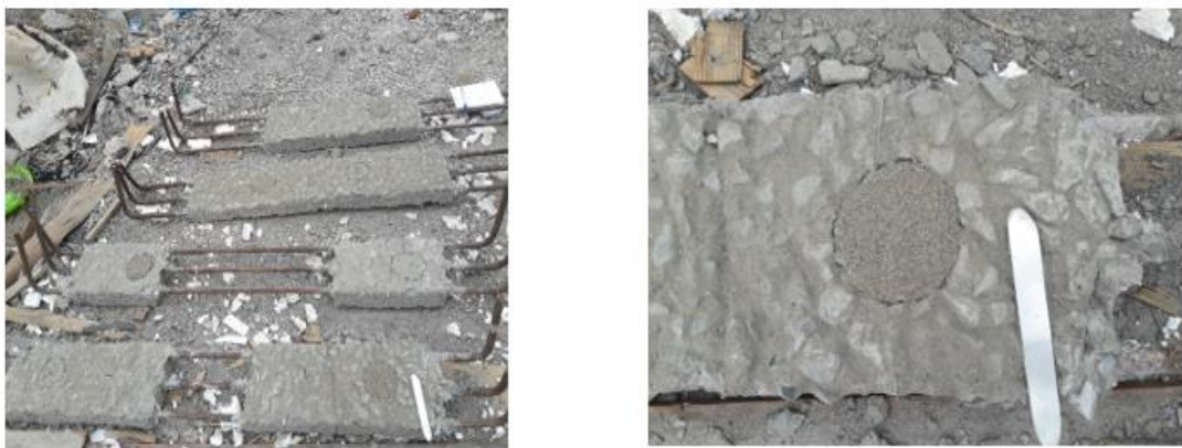
Figure 3-47 Patch selection of the sand patch test in damaged bond concrete sections
