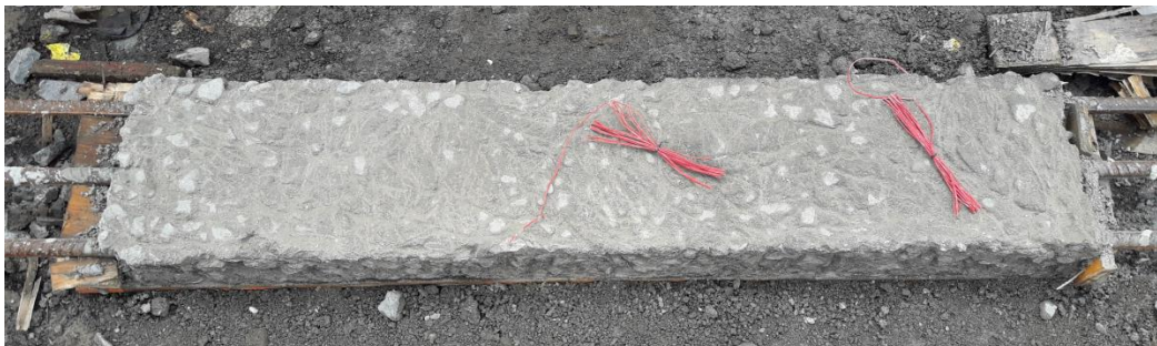
Figure 3-2 Rough surface formation
