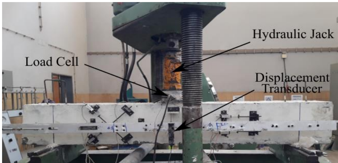
Figure 3-54 Test set up of the tests
