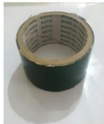
Figure 3-6 Materials used for bond cutting in pullout test
