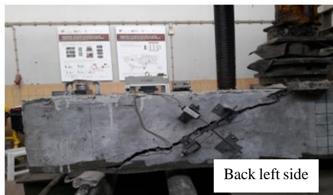
Figure 5-27 Close up on the cracks and spalling of beam 75DCB2
