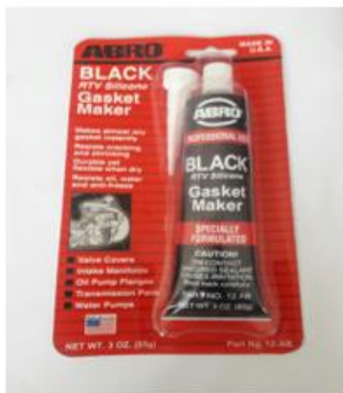
Figure 3-6 Materials used for bond cutting in pullout test
