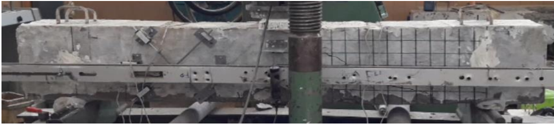
Figure 5-22 Cracks just before failure beam 75DCB1
