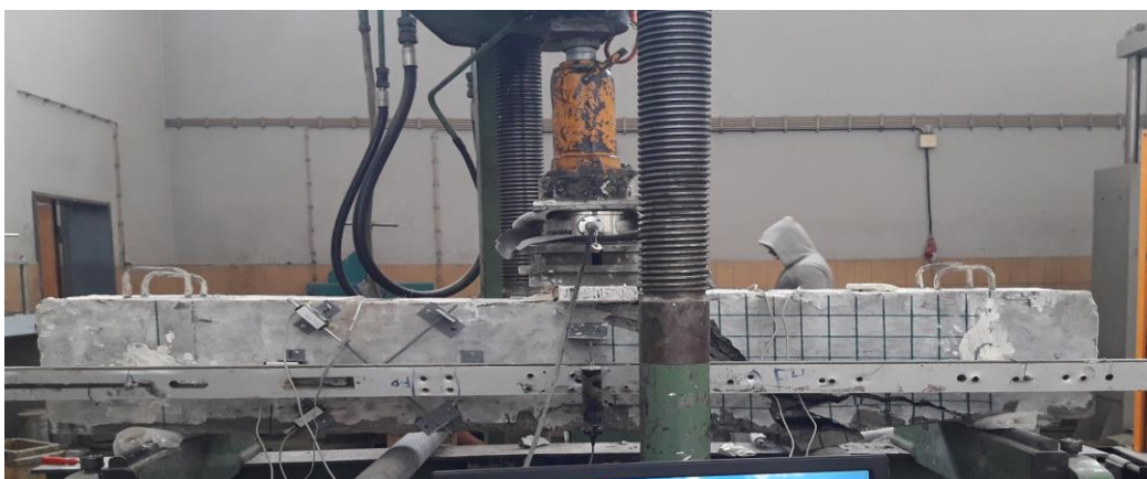
Figure 5-21 The beam 75DCB1 after failure
