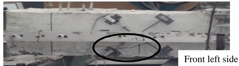
Figure 5-42 Control beam critical diagonal crack
