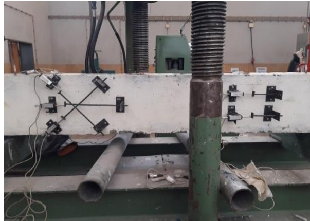
Figure 3-56 Surface measurement instrumentation set up of the trial beam
