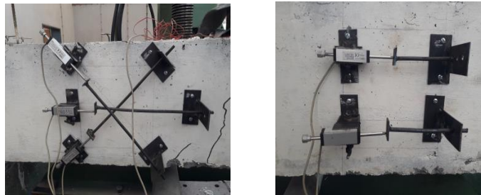
Figure 3-56 Surface measurement instrumentation set up of the trial beam
