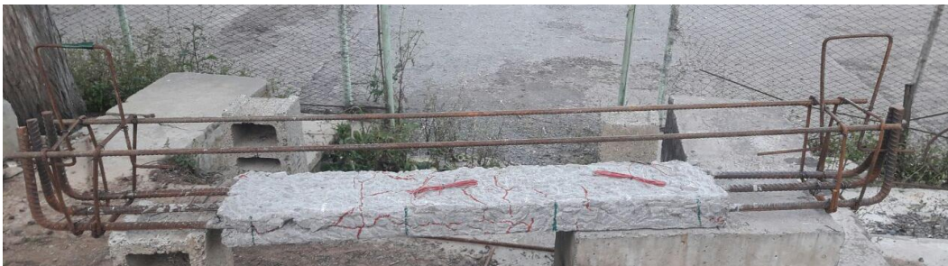
Figure 3-35 Trial beam damaged concrete section loading procedure
