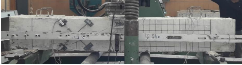
Figure 5-9 Cracks just before failure beam 75BB1
