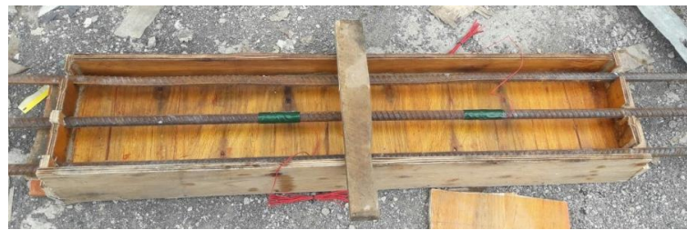
Figure 3-32 Form work for trial beam damaged concrete section
