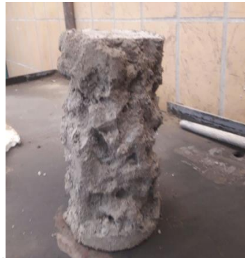
Figure 3-2 Rough surface formation
