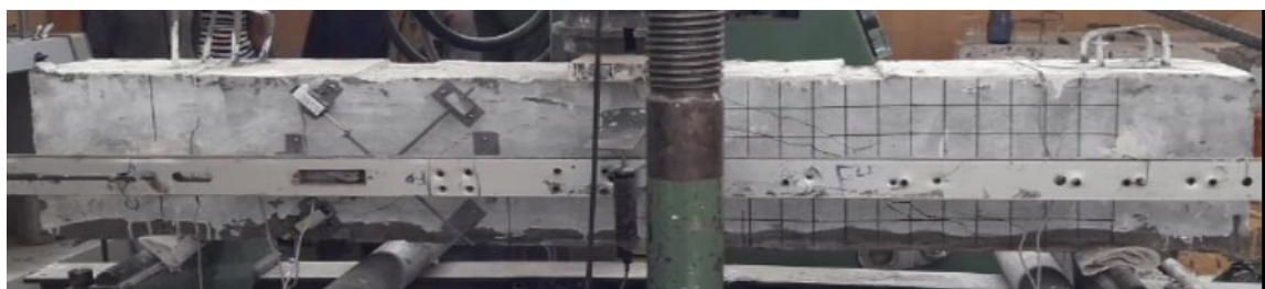
Figure 5-25 The beam 75DCB2 after failure
