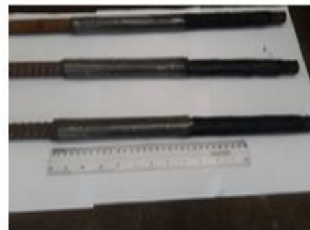
Figure 3-6 Materials used for bond cutting in pullout test
