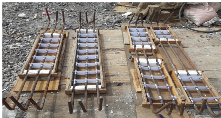
Figure 3-42 The bond deterioration imitation by winding water proof tape
