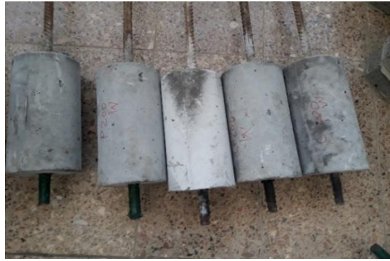
Figure 3-8 The pull out specimen
