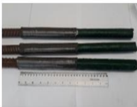
Figure 3-6 Materials used for bond cutting in pullout test
