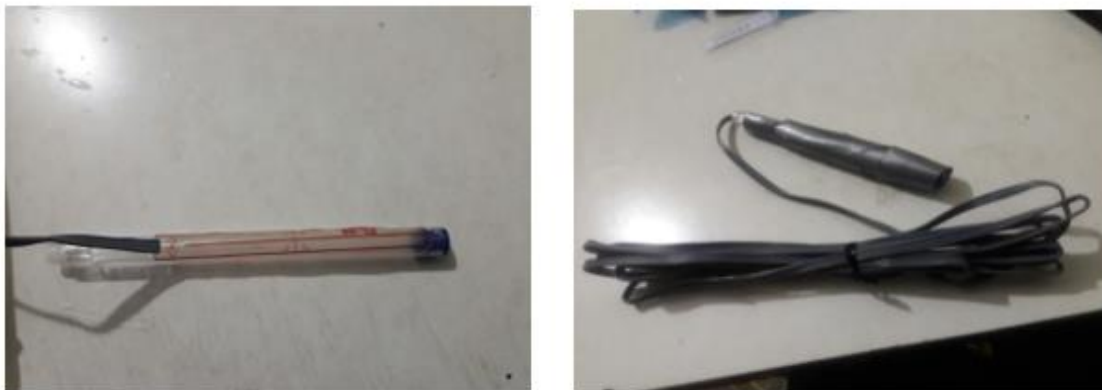
Figure 3-49 Fashioning of the mold strain gage
