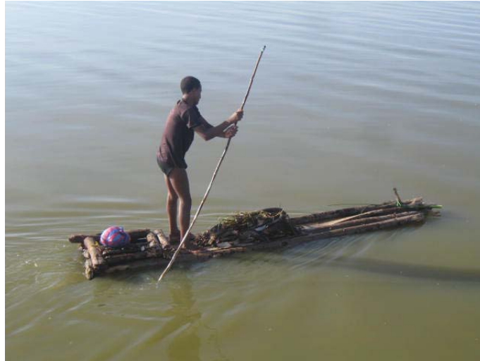
Figure 10: A traditional boat that is built up from zəgba , want'ε 'Cordia Africana' and bah'ir zaf 'Eucalyptus citriodora Hook' plants
