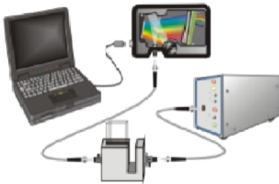
Figure 4.4: Ocean optics spectrophotometer set-up.
