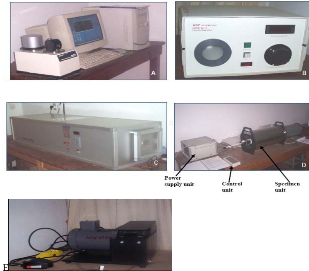
Fig.2.3Paleomagnetic Instruments used in laboratory.A)Spinner magnetometer. B) Impulse magnetizer. C) Thermal demagnetizer. D) alternating-field demagnetizer. E)Cutter.
