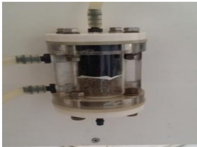
Figure 3.2 Arrangement of the fixed bed.
