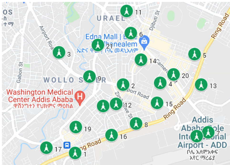
Figure 6.1: An operational LTE network with 21 eNBs (in total 63 sectors) around Bole area in the city center of AA.
