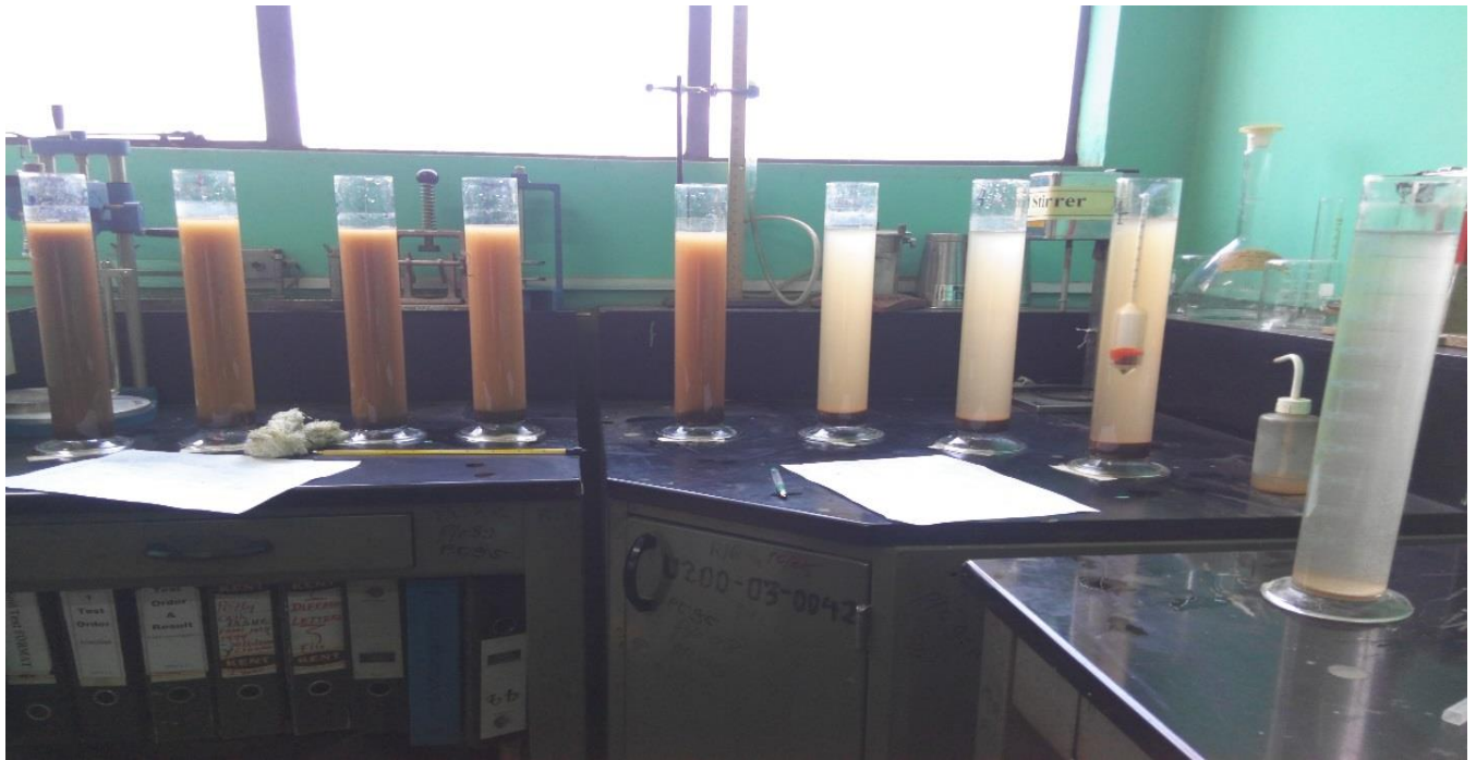
Figure 4-9: dispersion potential determination with different percentage of gypsum
