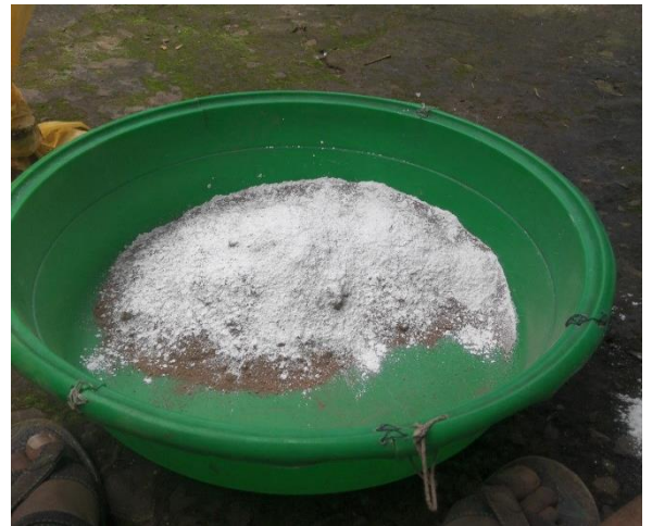
Figure 4-6: mixing dispersive soil with gypsum
