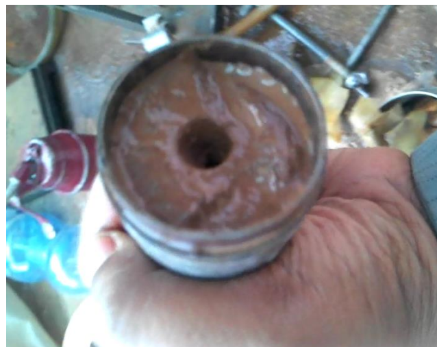
Figure 4-3: leached soil at the front face
