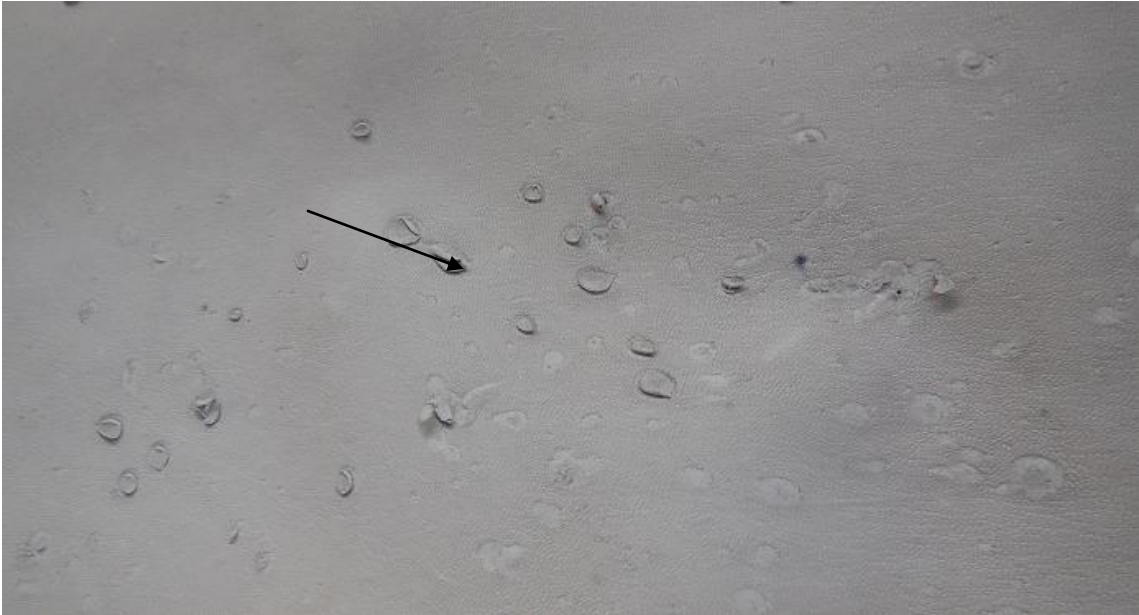
Figure 7: Processed skin at crust stage with defect due to pox (skin of sheep at fig.6)
