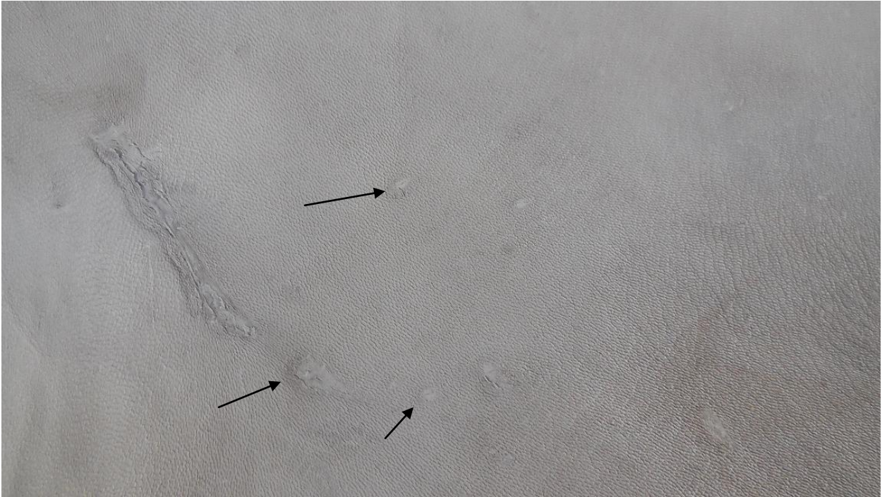
Figure 9: Defects on processed skin at crust stage due to flea infestation (from fig.8)
