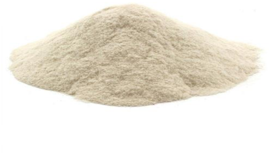
Figure 3.5 powder keratin protein after drying and grinding
