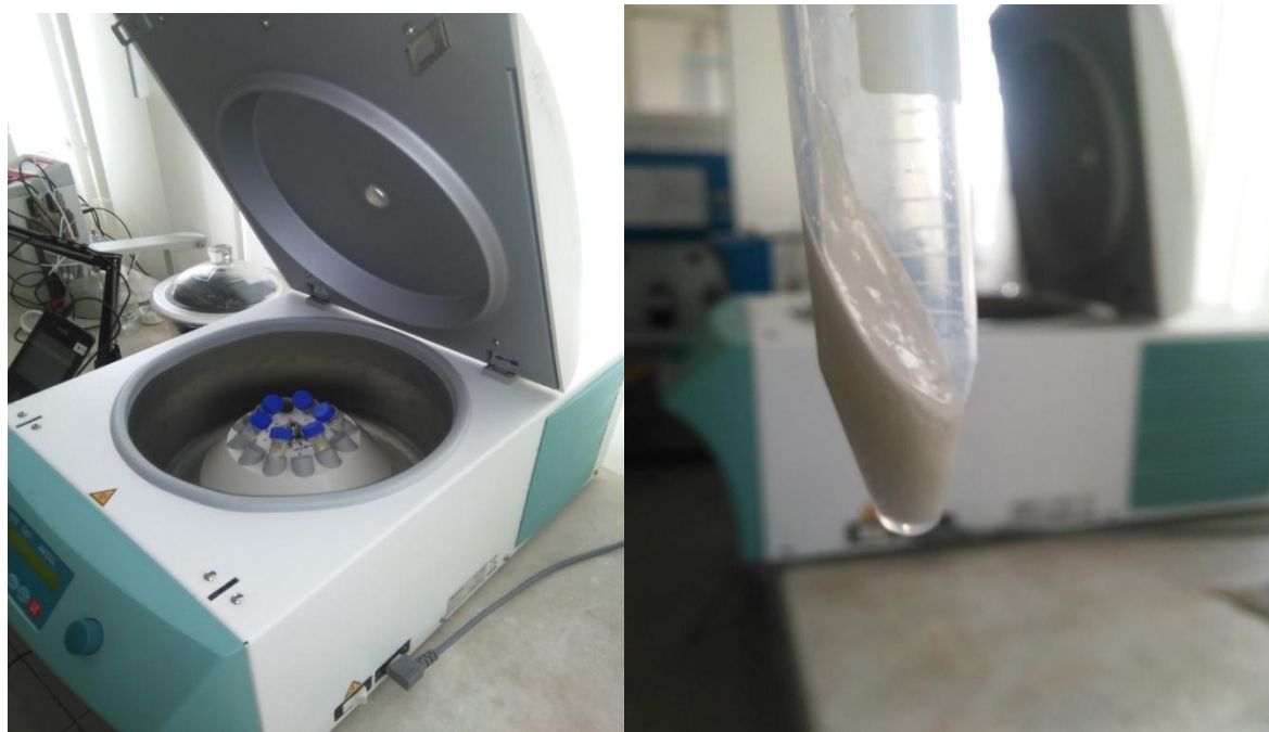
Figure 3.4 Centrifugal separation (Left) and separated keratin protein inside test tube (right)
