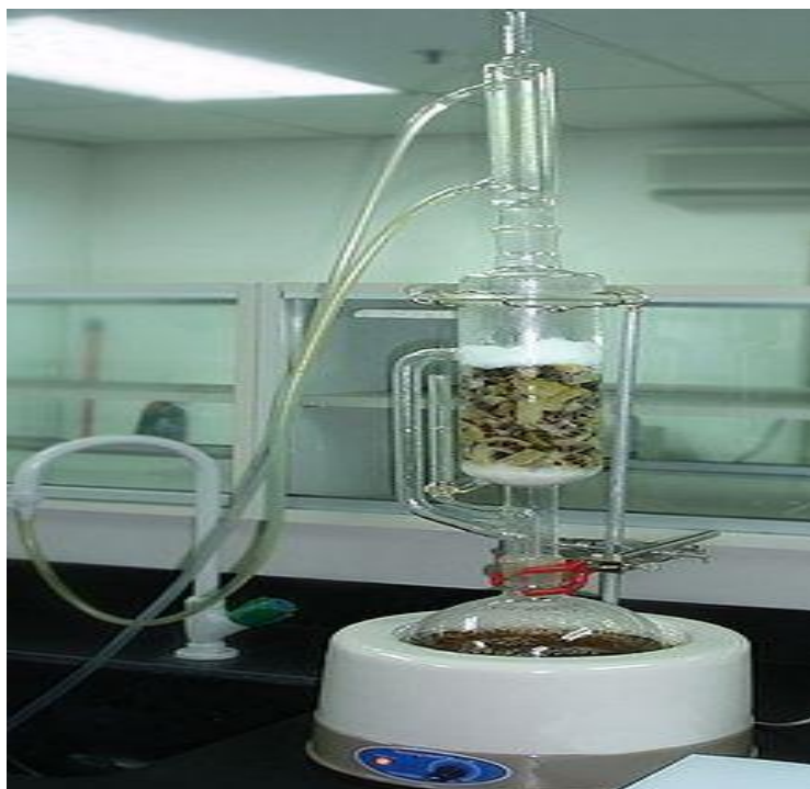
Figure 3.1 Setup of the Soxhlet Apparatus
