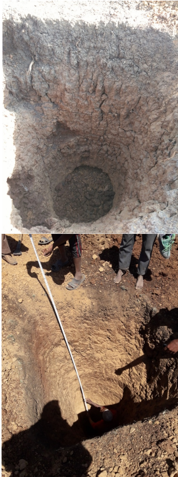
Plate 5 - 1: Different layers of Germama clay in test pit KDCL-01 and KDCL-02
