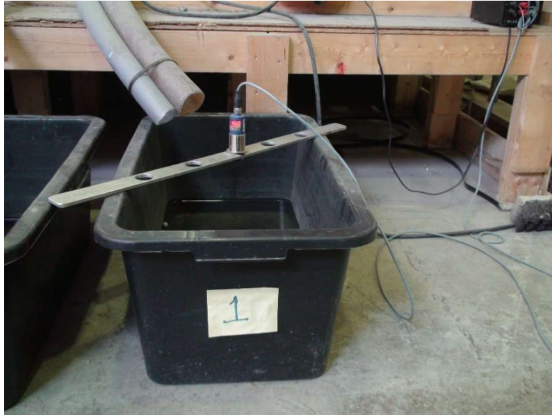
Figure 24: Ultrasonic sensor used for measuring the overtopping volume over the dam crest in each bucket.
