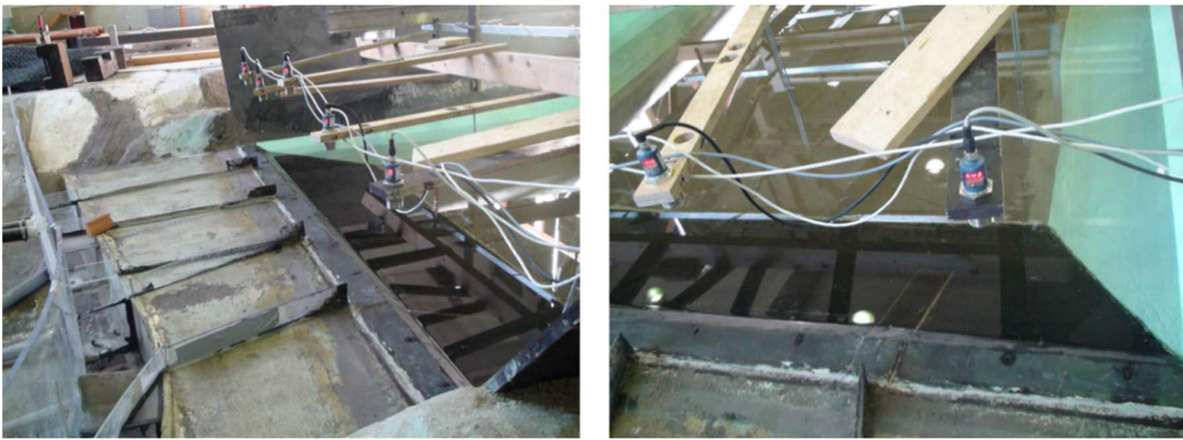
Figure 23: The picture of five ultrasonic sensors for measuring the overtopping depth along the five dam crest sections.
