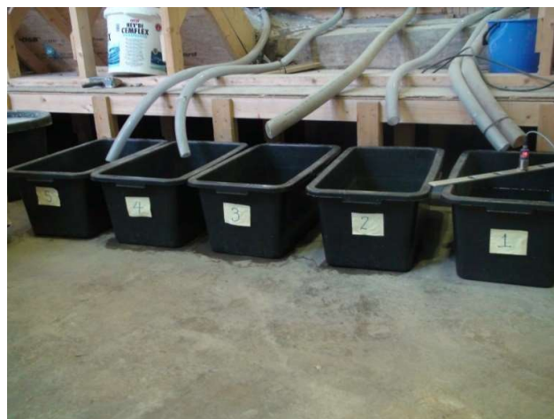
Figure 21: Picture of the five buckets collecting the overtopping water over the five dam crest sections.
