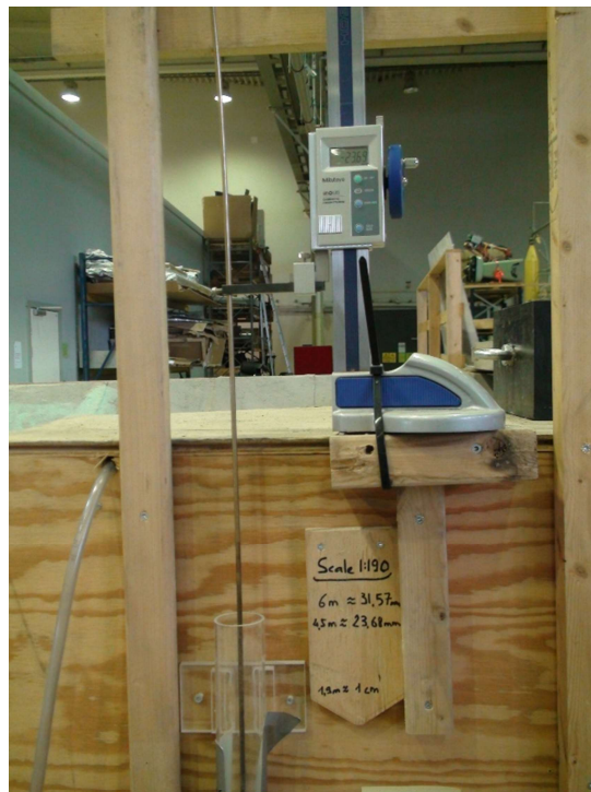
Figure 27: Picture of a Piezometer used for measuring the reservoir water level.
