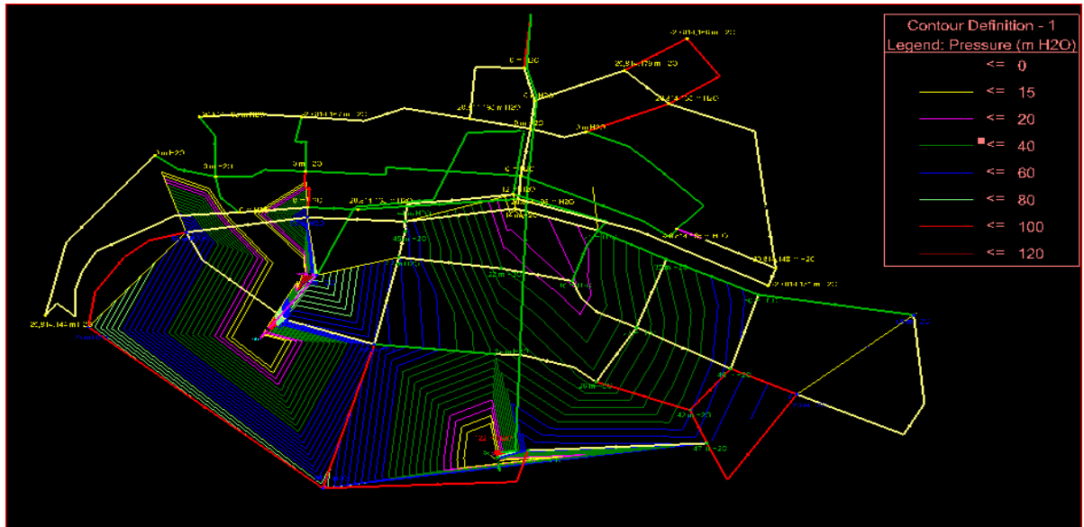
Figure 4-12: Pressure contour at Peak hour-2 Day Demand (15:00 hr.)
