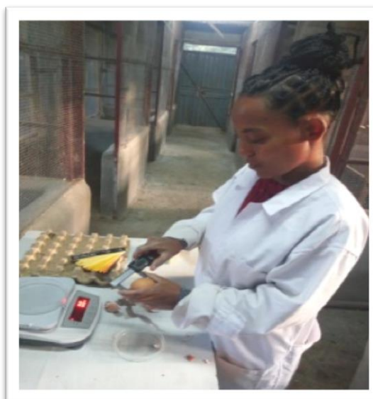
Figure 3: Egg width (left) and length (right) measurement using digital caliper
