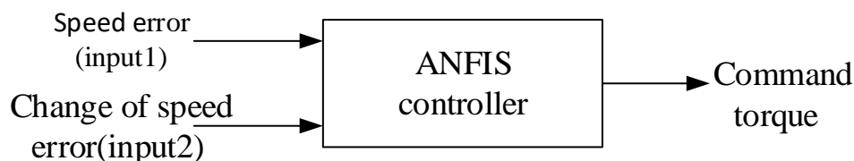
Figure 3.16 Input/output of ANFIS controller
