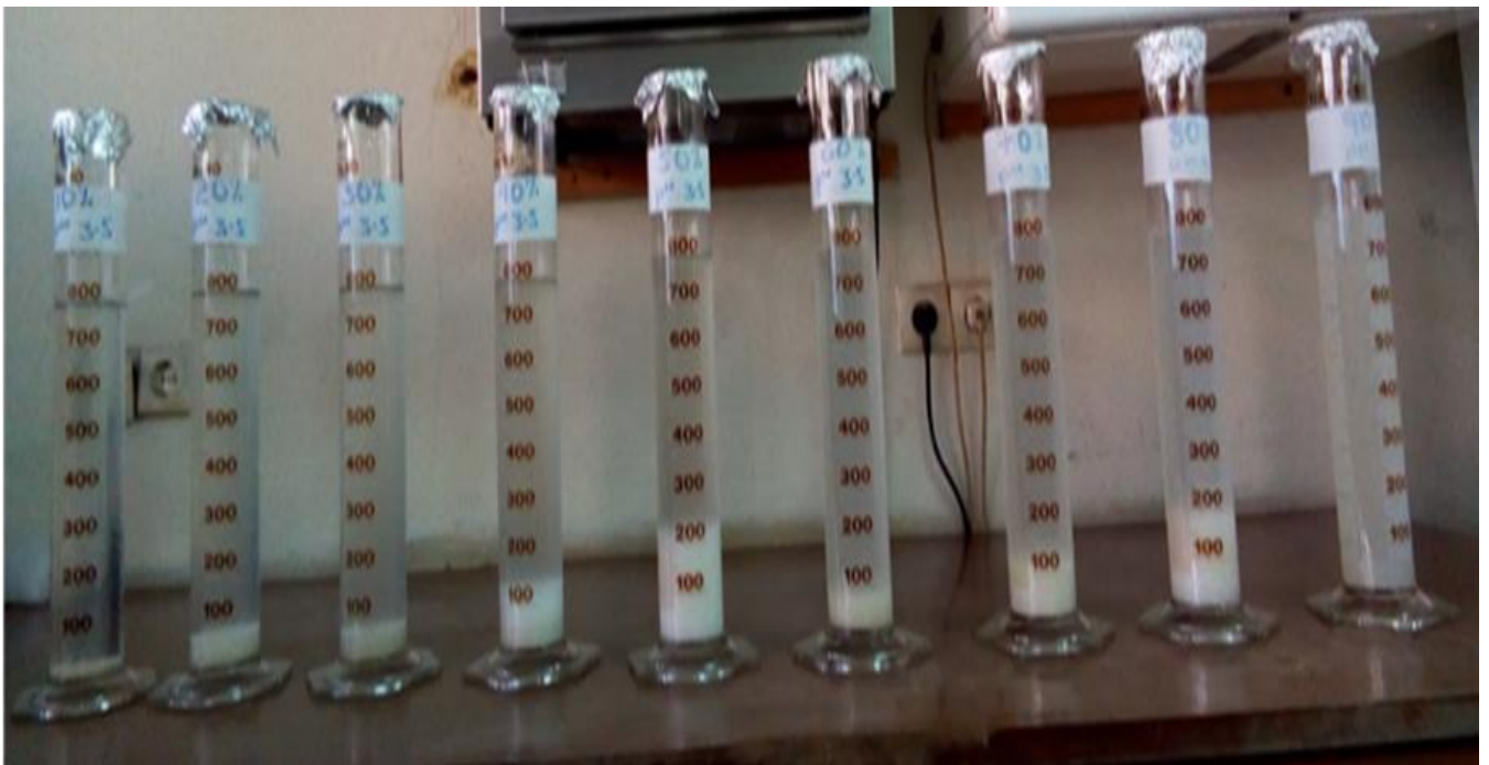
Fig 3.1b Pictures of coacervates prepared at pH 3.5 and 10/90 to 90/10 sodium alginate/gelatin B polymeric ratio
