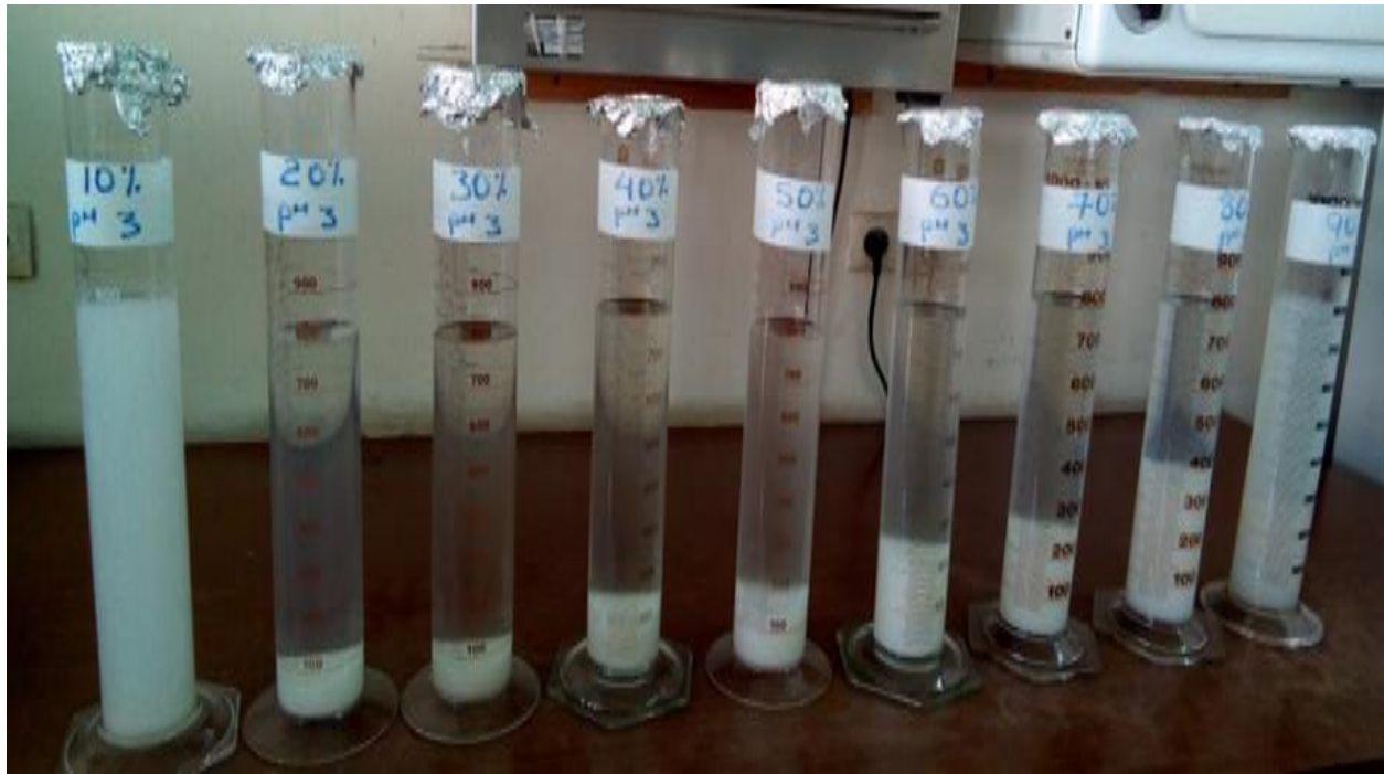
Fig 3.1a. Pictures of coacervates prepared at pH 3 and 10/90 to 90/10 sodium alginate/gelatin B polymeric ratio
