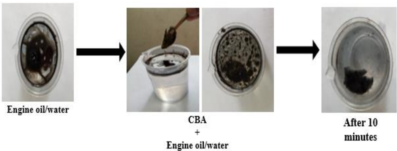
Figure 18: Test for Engine oil removal from waste water using CBA
