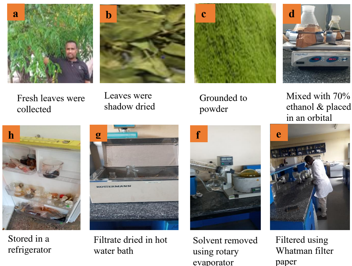
Figure 5: Plant material preparation and extraction using 70% ethanol
