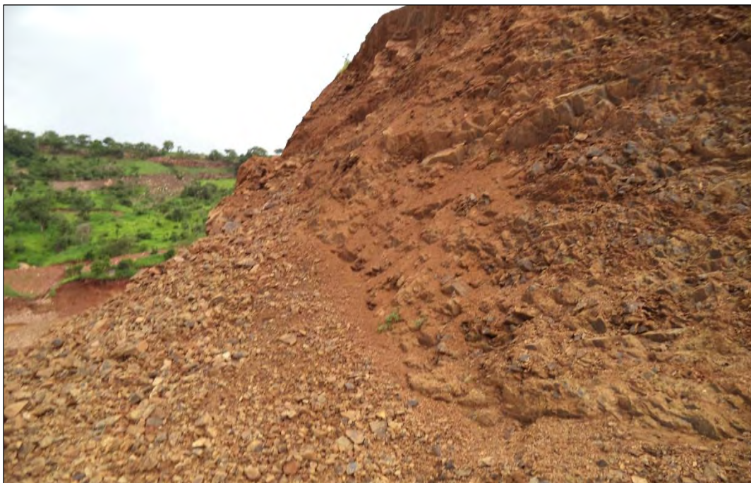
Plate 5.2: Rock mass failure occurred in highly fractured and weathered rocks of the study area
