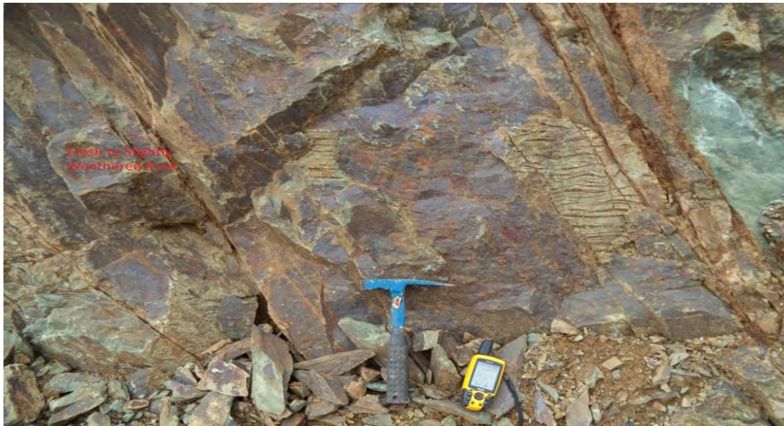
Plate 4.3: Fresh to slightly weathered and widely jointed rock masses in the study area
