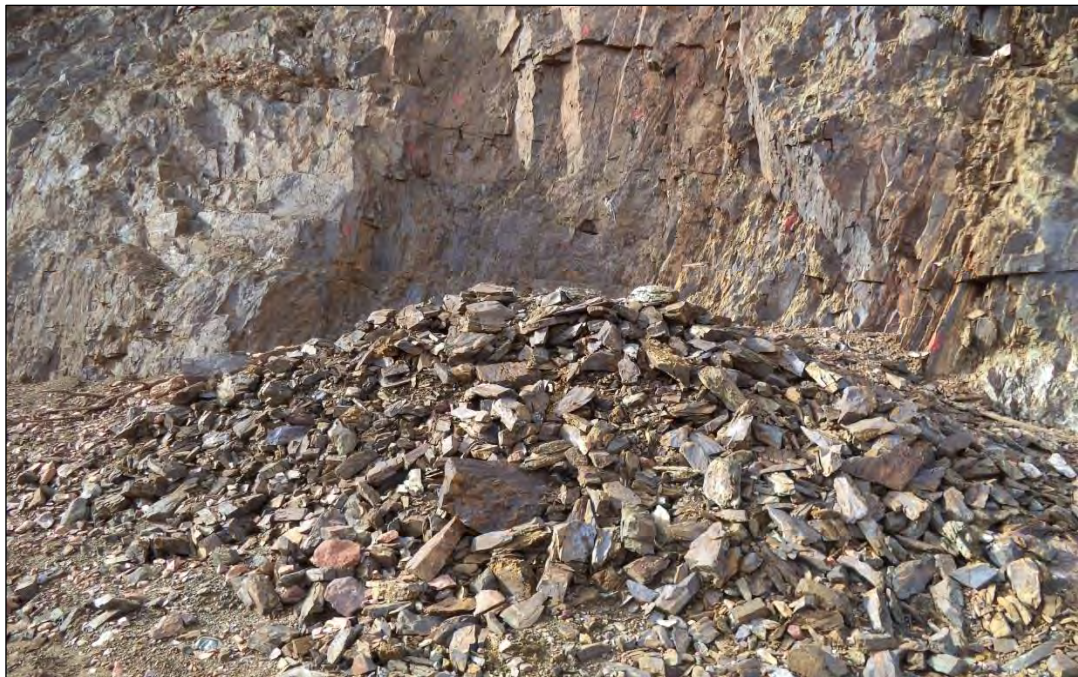
Plate 5.1: Rock mass failures occurred in the study area due to crosscutting relationships of the joint structures
