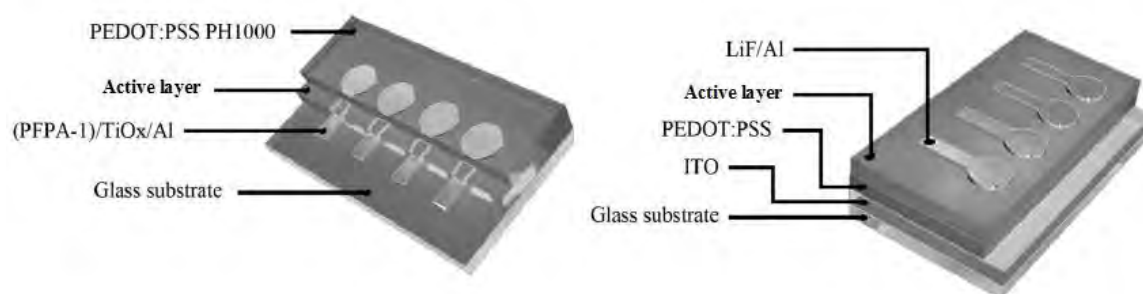
Figure 3.1.4. Device architecture of inverted (left) and conventional (right) solar cell devices [200].
