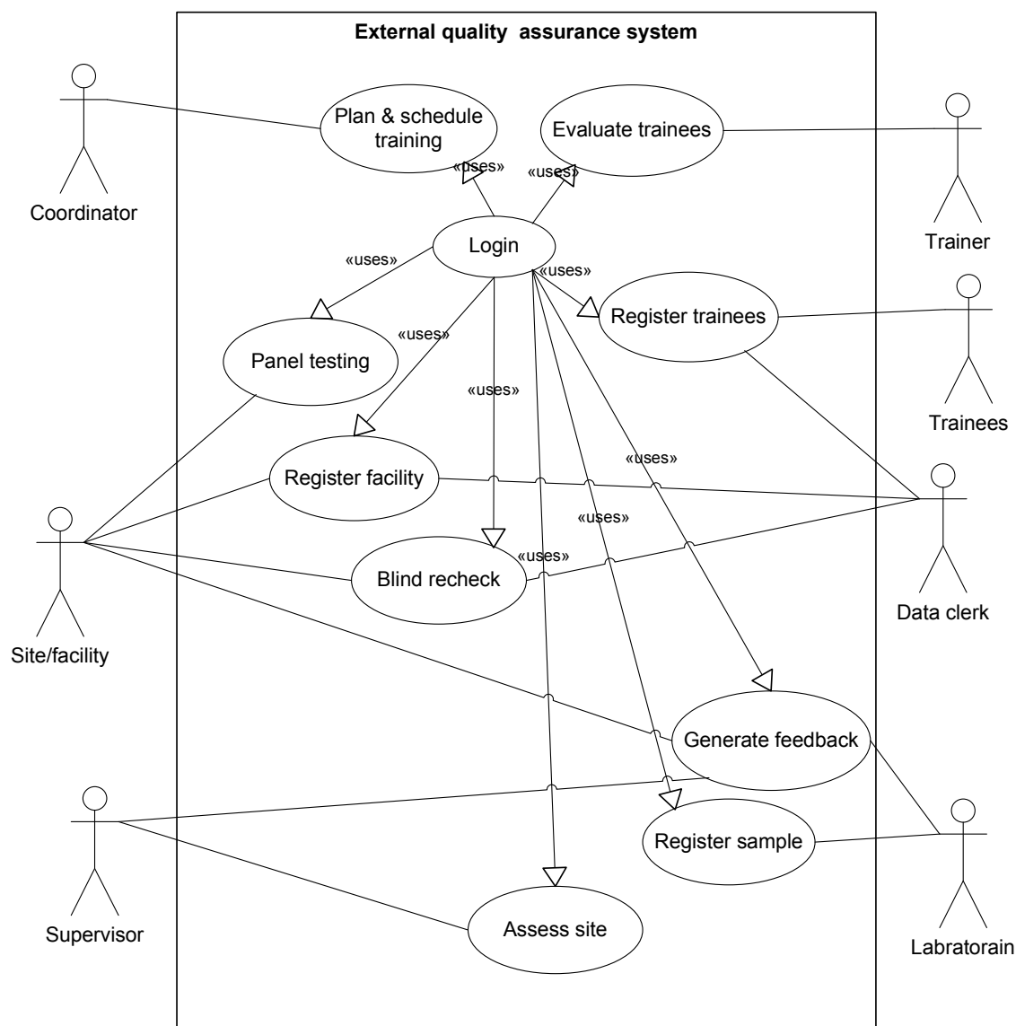
Figure 4-10 use case diagram of new EQA system
