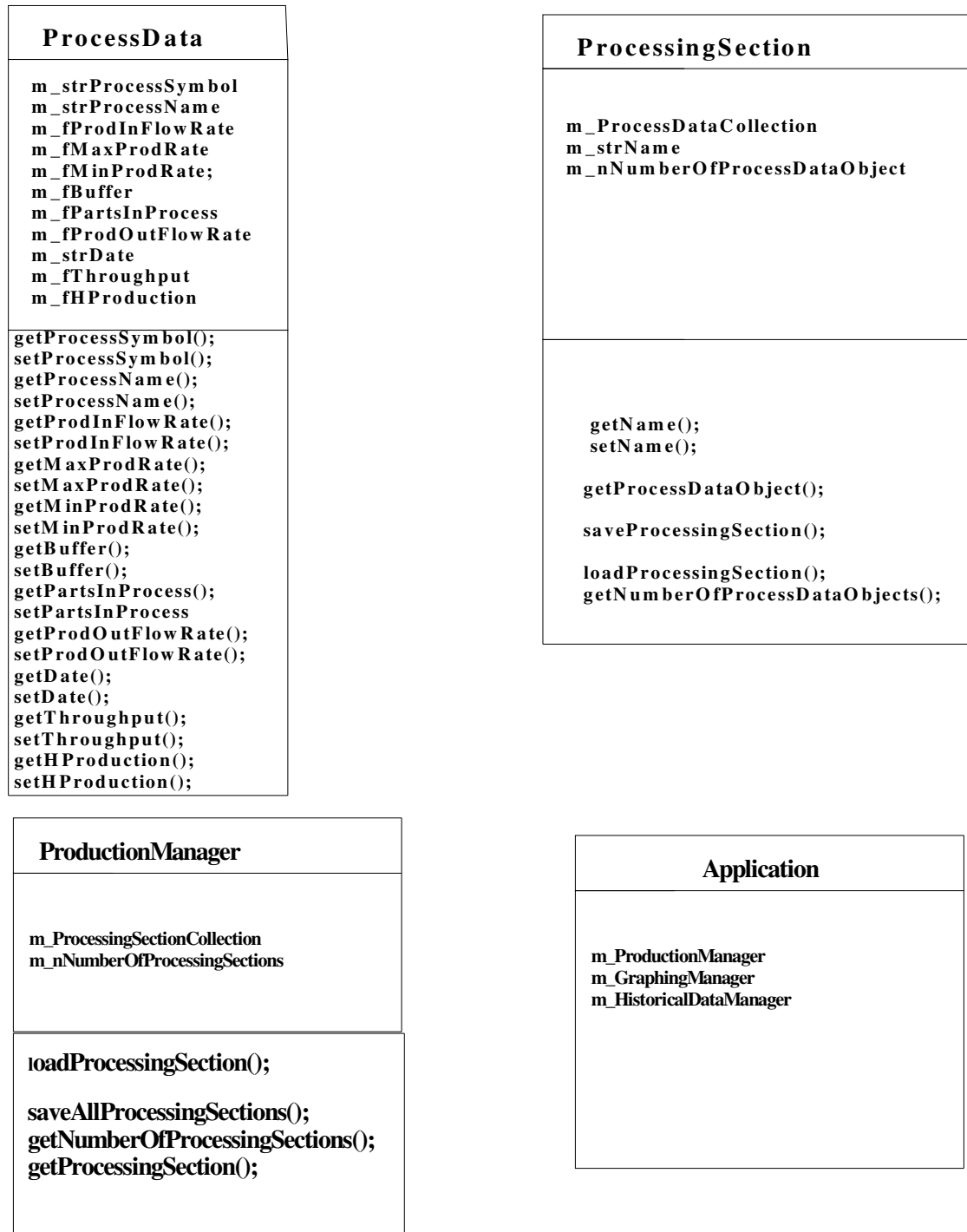
Figure B-1 Class definitions of potential object classes in the developed software
