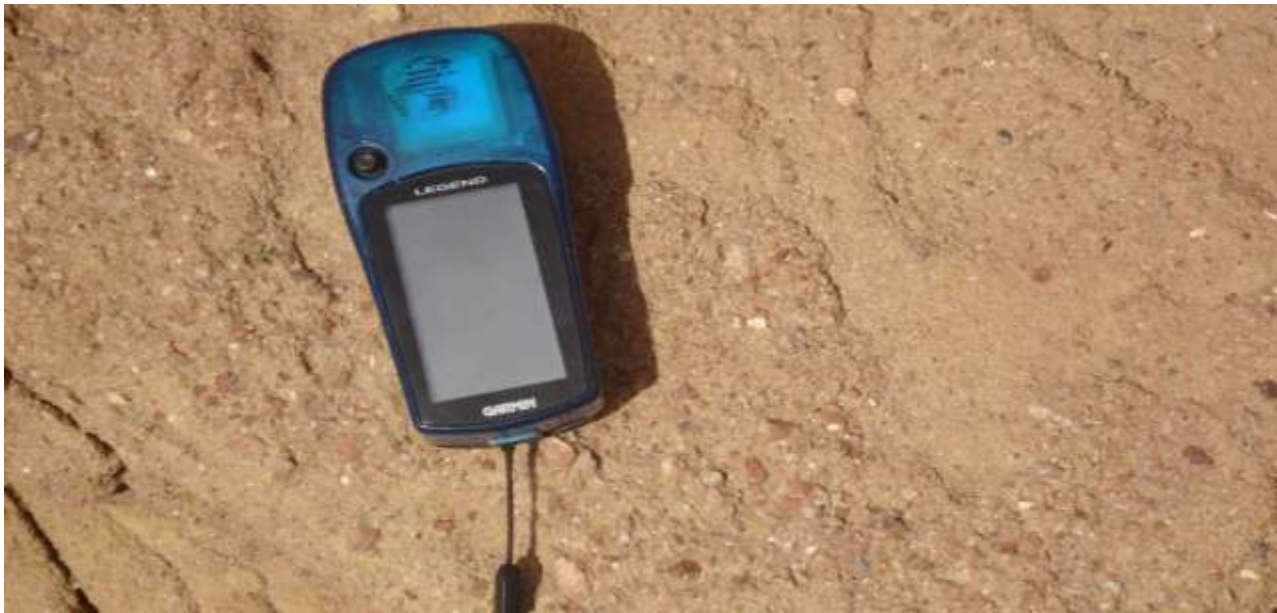
Figure 3.9 GARMIN Hand held GPS used to collect Ground Truth data in the Field.
