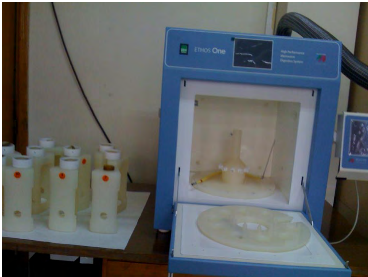
Fig.3.5 ETHOS One Micro wave Digester (EPHI laboratory)
