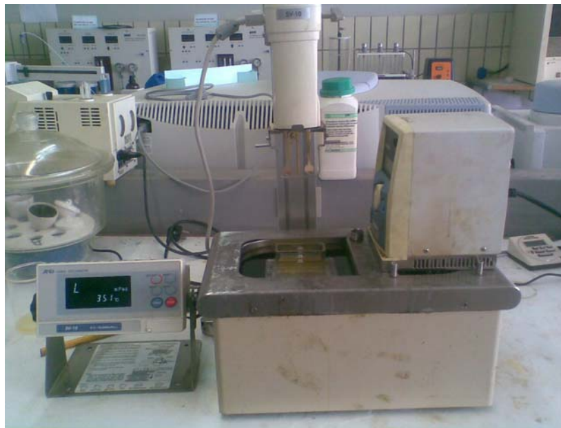
Fig 3.8 Experimental set-up for viscosity determination
