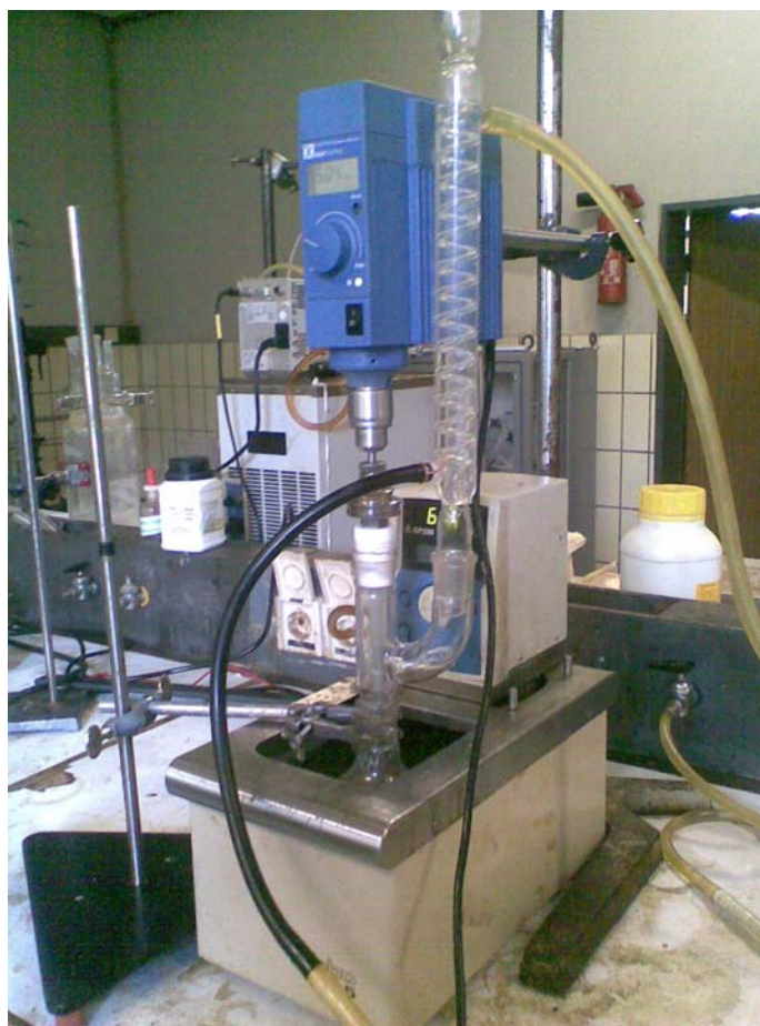
Fig. 3.7 Experimental set-up for biodiesel production through transesterification
