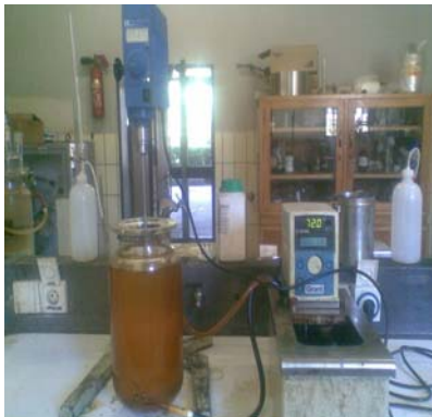
Fig. 3.5 Experimental set up during degumming process for purification of crude Jatropha oil
