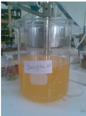
Fig. 3.4: Crude Jatropha Curcas oil collected during extraction process
