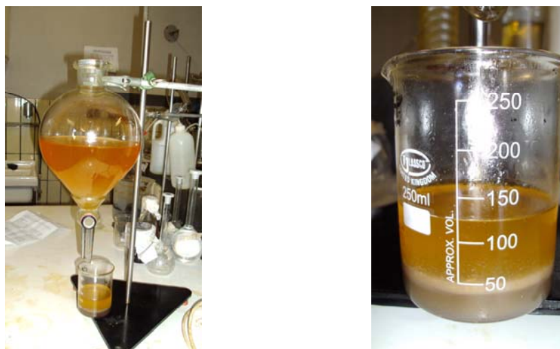
Fig.3.6 Jatropha oil after Degumming on settling tank to separate the white and dark precipitates
