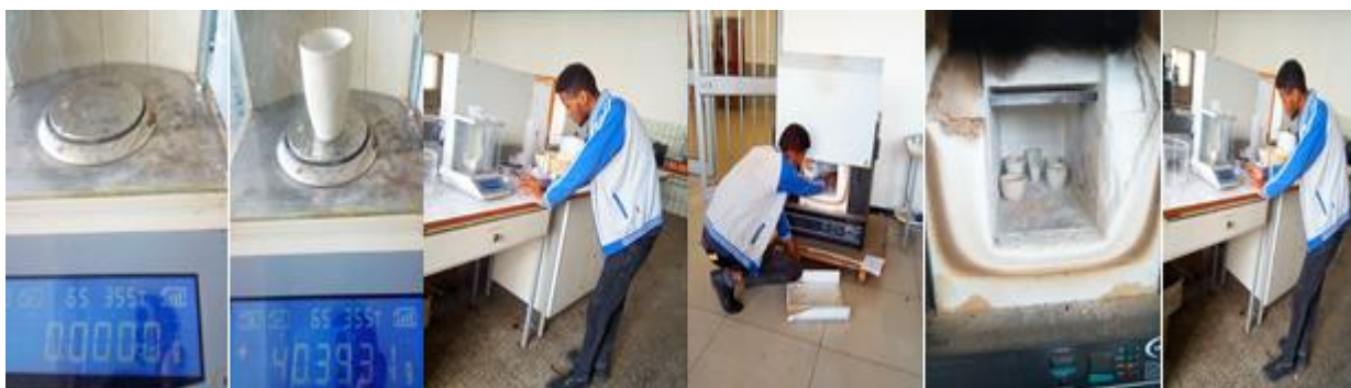
Figure 12: Measuring ash and moisture content.
