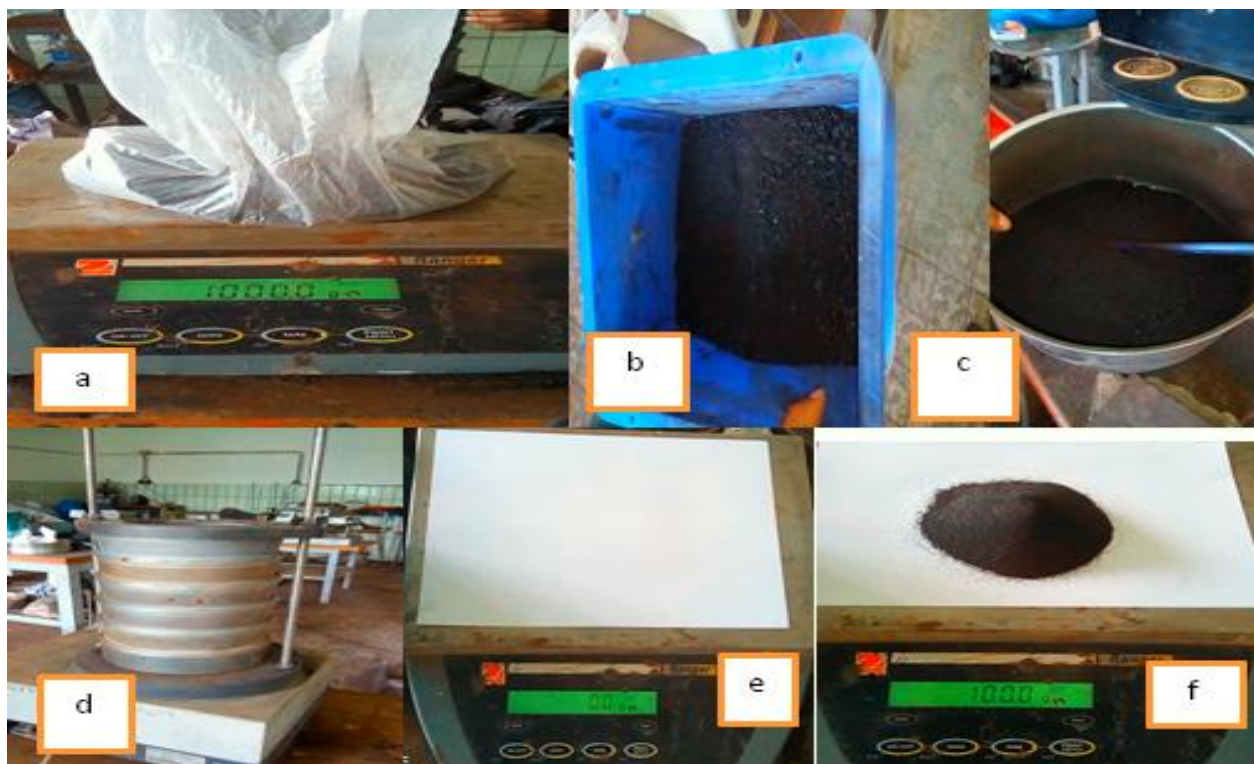
Figure 8: Preparation of samples shows 1kg coal for crushing, b) sample after crushing, c) sample after grinding, d) sample during screening, e) checking balance/instrument/ before adding the sample it must be 0.0g and f) 100.0g of prepared sample for further analysis.
