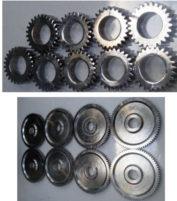
Figure 3.9:- Manufactured gears and pinion before application of fault
