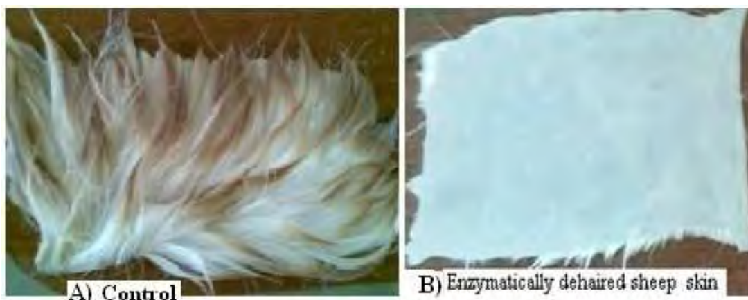
Figure 20: Complete dehairing activity using 58U/ml alkaline keratinolytic protease produced by Vibrio sp. without any addition of lime and sodium sulfide in the reaction mixture at 37°C for 12h incubation A) Sheep skin with heat-denatured alkaline enzyme at 100°C for 1h, with buffer (control) and B) Enzymatically dehaired sheep skin incubated with non-denatured enzyme.
